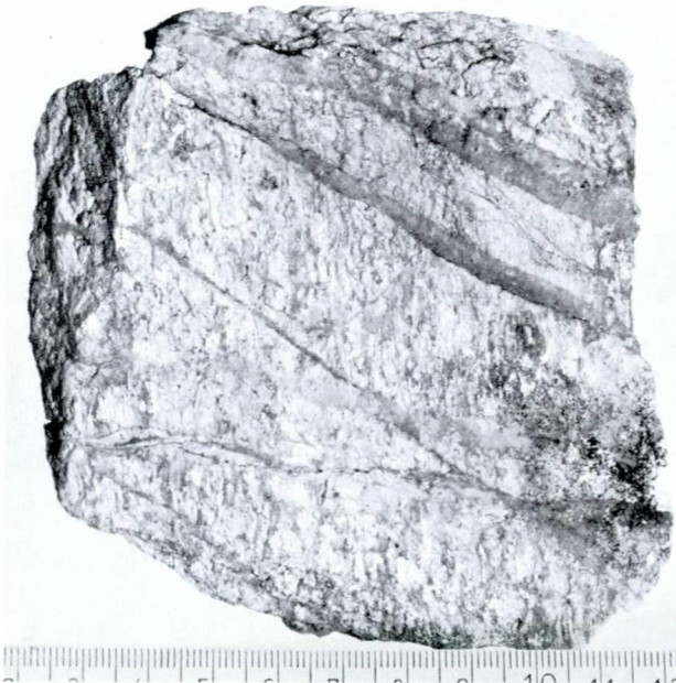
Fig. 9. Granitic augen gneiss with a stockwork of quartz-molybdenite veinlets from the Aurtjern area in Skrukkelia. Scale in centimetres.
