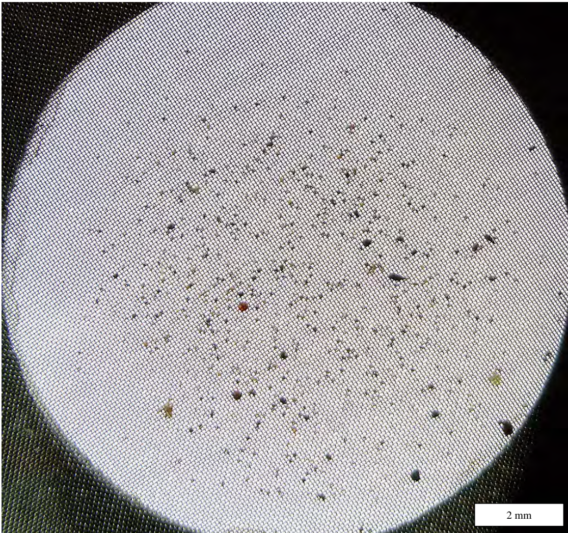
Figure A2.10 Sample S-04 (0-2 cm), filter 2. Mostly PE and PE-chlorinated, some nylon, PE:PP, melamine particles. Photo taken in bright field mode.
