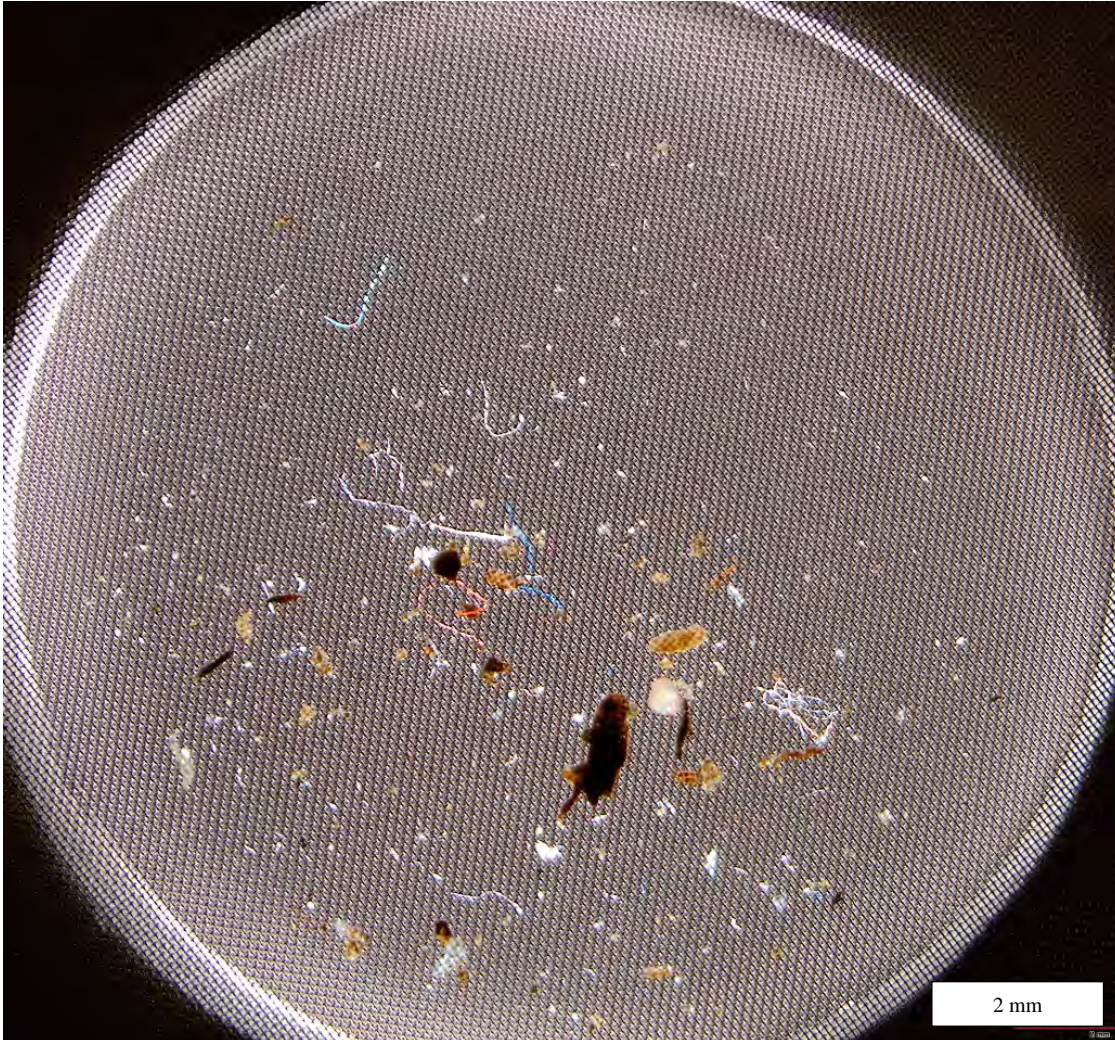
Figure A1.15 Method blank MB-16. Mostly PTFE and PE. Photo taken in polarized mode.
