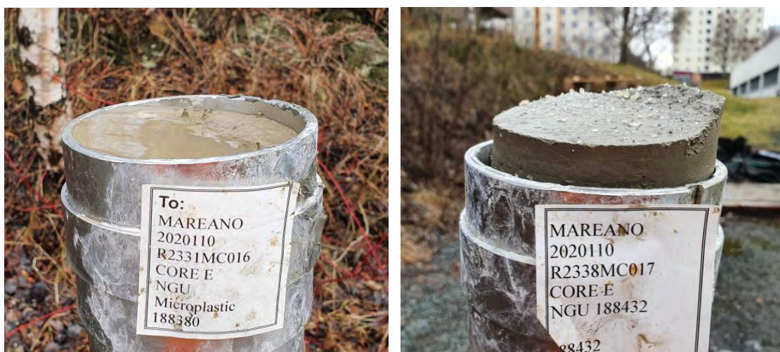
Figure 1 Sediment cores sampled for microplastic analysis in steel tubes, showing a core where seawater is intact (left) and where seawater has leaked out during storage/transfer (Photos from NGU).
