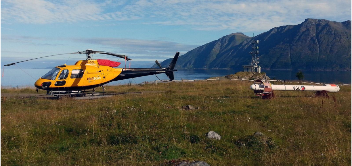
Figure 2: HeliScan helicopter and Hummingbird system on the ground in Ystneset, Øksfjord
