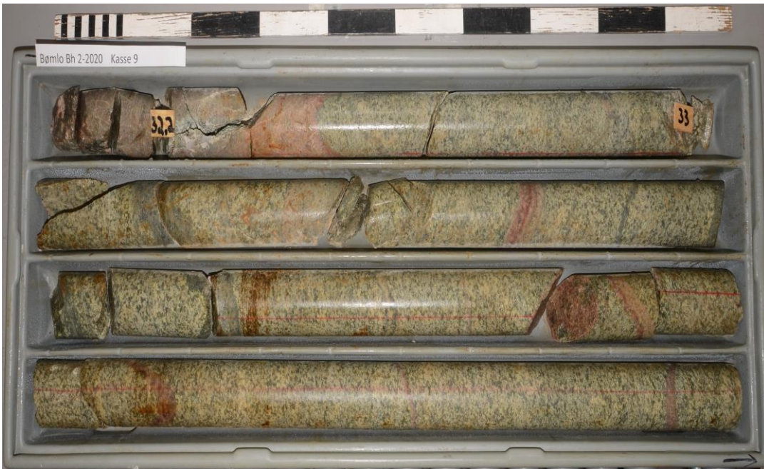
Figure 74. Bømlo Bh2. Soft rock at 25 m (upper) and hard rock from 32.5 m (lower).
