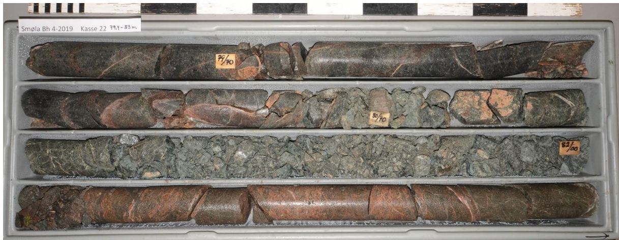
Figure 26. Bh4, Smøla. Cores 79.4 – 83.0 m depth.
