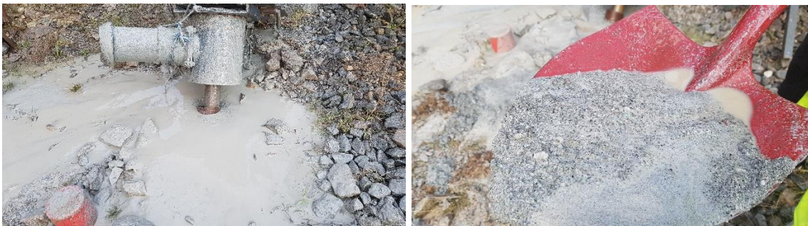
Figure 109. Clay and sand from the fracture zone at 24 – 26 m in Bh2
