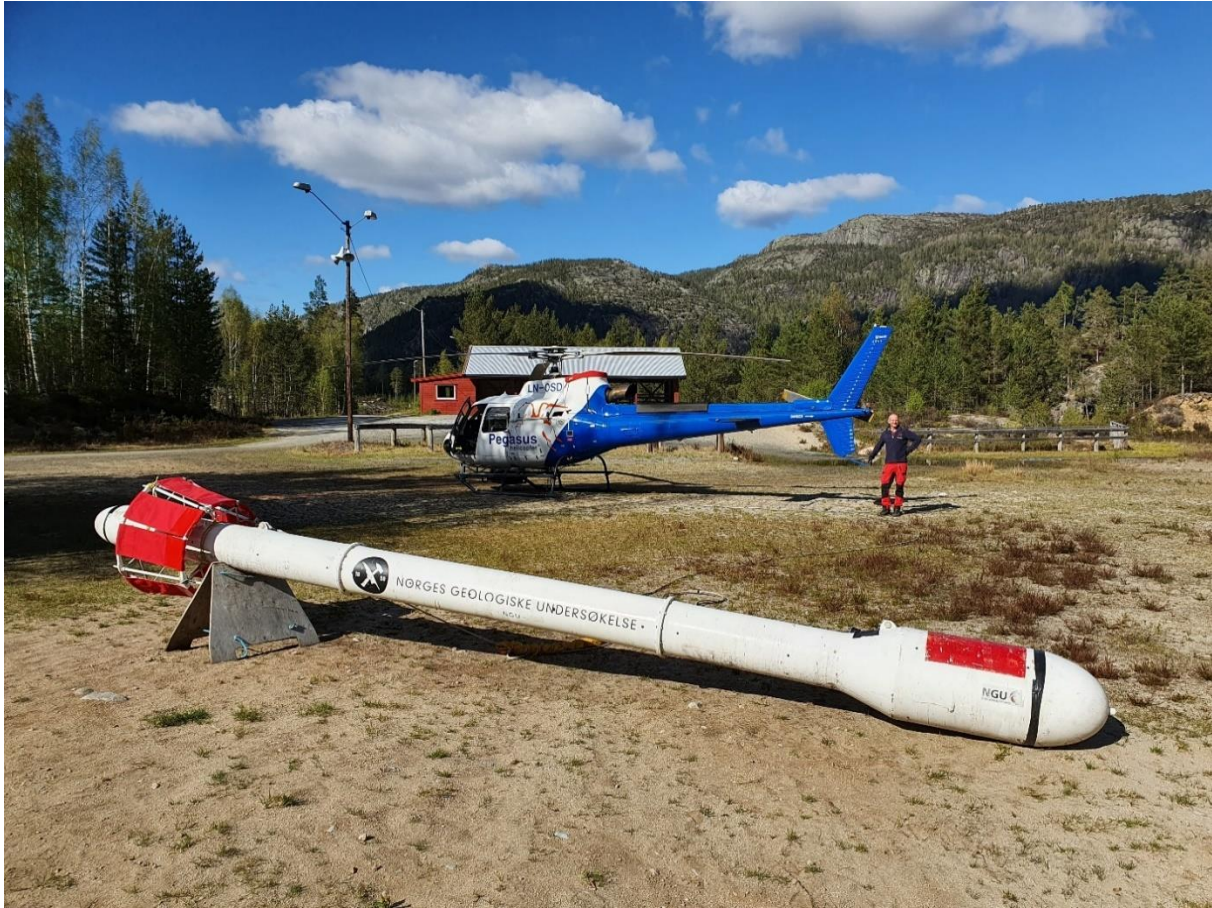
Figure 2: Pegasus helicopter with pilot and NGU Hummingbird EM system
