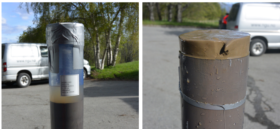
Photo 1 Overview of sealed sediment core in PVC tube (left) and detail photo of surface sediment (right).
