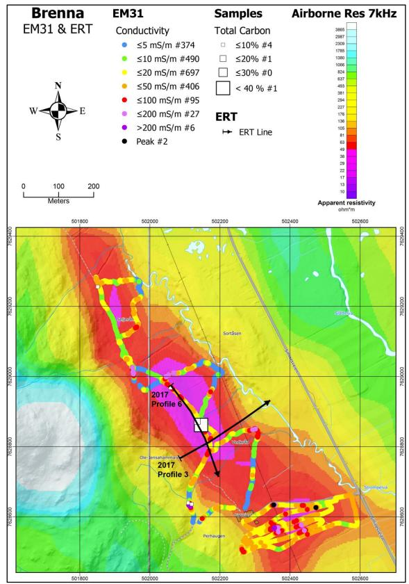
Figure 7.2: The Brenna area. The results from the EM31 measurements superposed on apparent resistivity (EM 7 kHz coaxial coil configuration, Rodionov et al. 2013a). Black lines show the locations of ERT/IP profiles. The locations of graphite samples and their TC content are shown as white squares.
