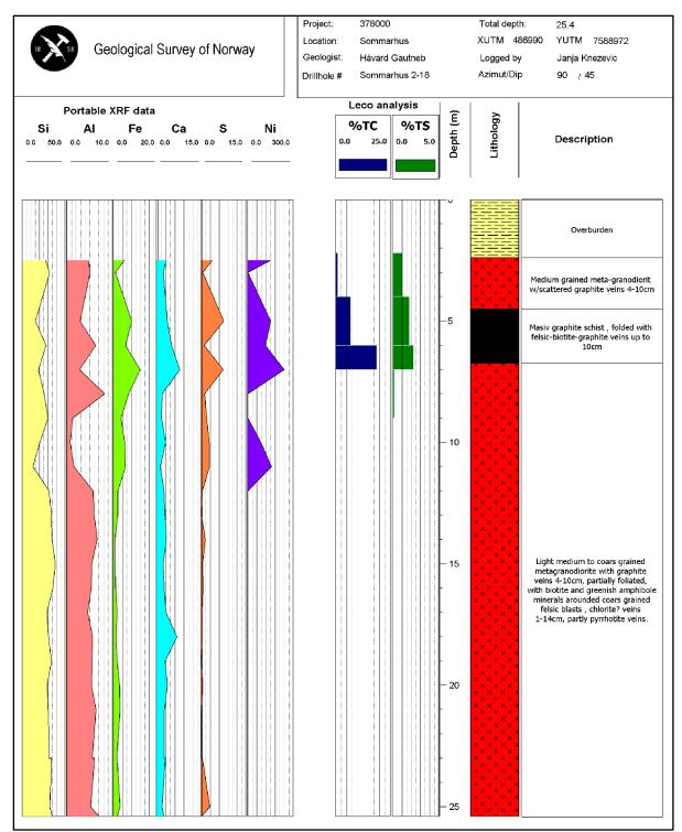
Figure 9.12: Results from the Sommarhus drill-hole Dh2-2018: Portable XRF analyses (Si, Al, Fe, Ca, and S in %, Ni in ppm) at the cores, selected Leco analyses of Total Carbon (TC) and Total Sulphides (TS), lithological log and core description.
