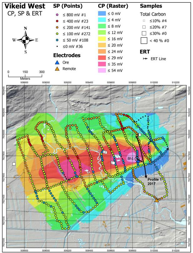
Figure 7.21: The Vikeid West area. SP data superposed on a contour map of the CP data. A black line shows the location of the ERT/IP profile. Locations of graphite samples and their TC contents are shown as white squares.
