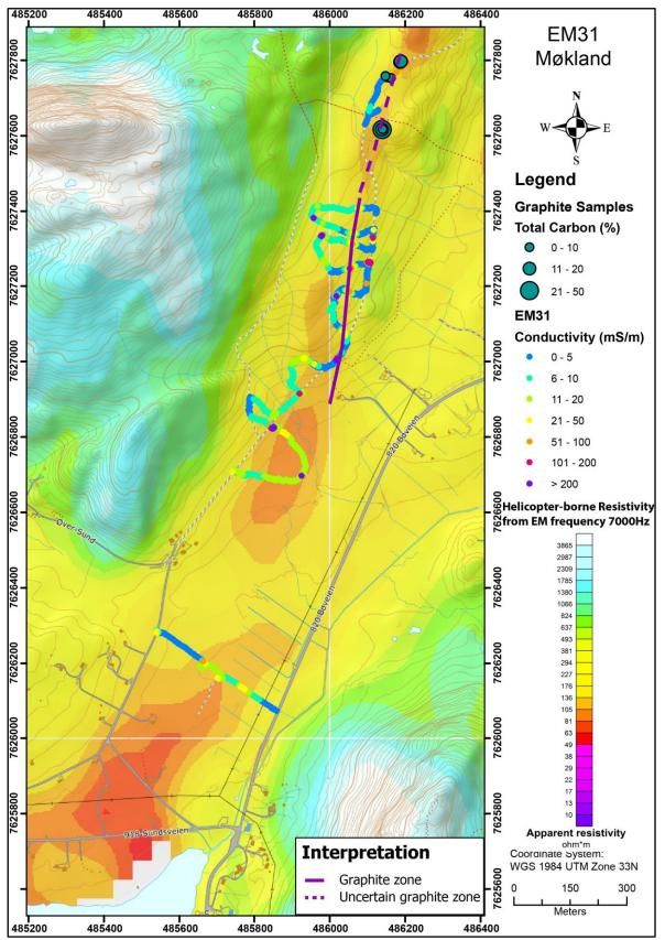
Figure 6.12: Results of EM31 measurements in the southern part of the Møkland area undertaken in 2017 superposed on apparent resistivity (7 kHz, from Rodionov et al. 2013a). Locations of graphite samples and their Total Carbon grade are shown with green circles (from Rønning et al. 2018).
