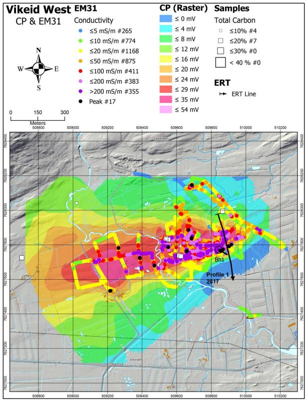
Figure 7.22: The Vikeid West area. The results from the EM31 measurements are superposed on the CP contour map. Locations of graphite samples and their TC contents are shown as white squares, the ERT/IP profile as a black line.
