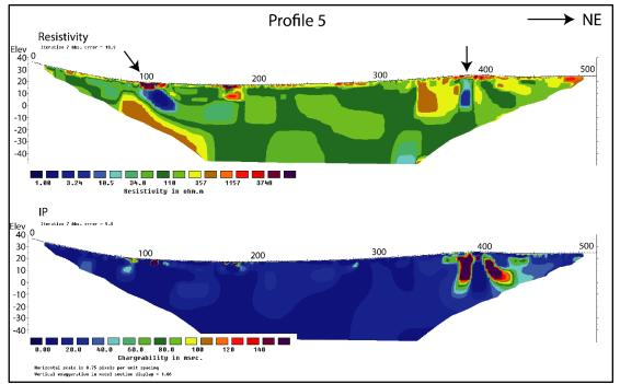
Figure 6.8: Olsetvatnet. 2D resistivity (top) and IP (bottom) results along profile 2018-5. No graphite outcrops are observed, but potential (interpreted) graphite zones are indicated with black arrows.
