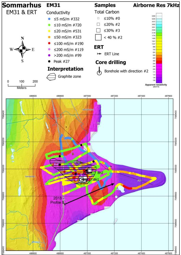
Figure 9.13: Sommarhus. An interpreted maximum extension of graphite based on helicopterborne EM and ground EM31 data. Both methods indicate good conducting material at the eastern peak of the Øyra peninsula. It is unclear whether this is caused by graphite or salt seawater in sediments.
