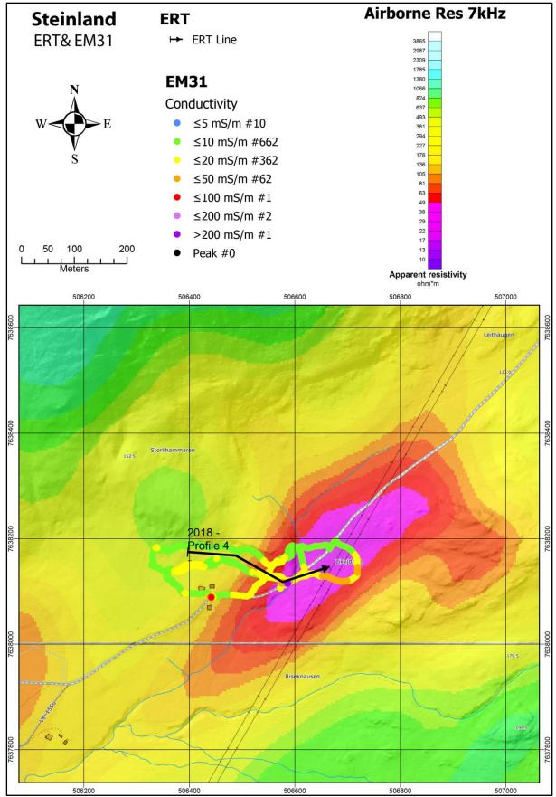
Figure 8.11: Results of EM31 measurements from the Steinland area overlain helicopter-borne measurements of apparent resistivity from EM 7 kHz coaxial coil configuration (from Rodionov et al. 2013a). The location of ERT/IP line is shown as a black line.
