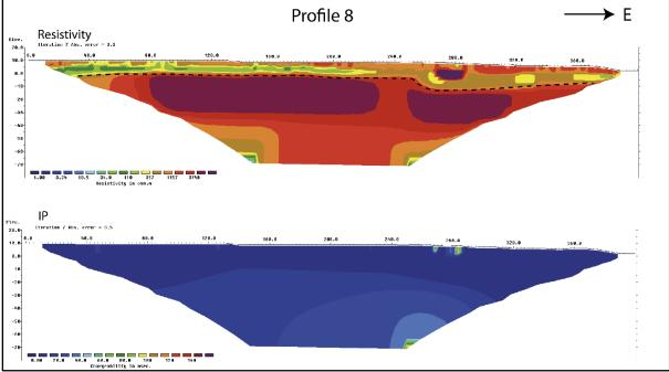
Figure 9.10: The Sommarhus area. The results of the 2D Resistivity and Induced Polarisation measurements along profile 2018-7. The interpreted soil-bedrock interface as dotted black line.
