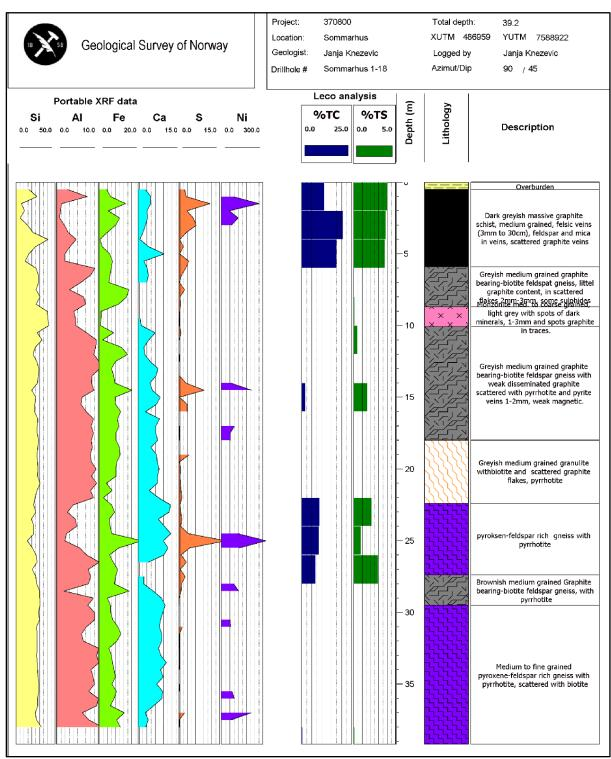
Figure 9.11: Results from the Sommarhus drill-hole Dh1-2018: Portable XRF analyses (Si, Al, Fe, Ca, and S in %, Ni in ppm) at the cores, selected Leco analyses of Total Carbon (TC) and Total Sulphides (TS), lithological log and core description.
