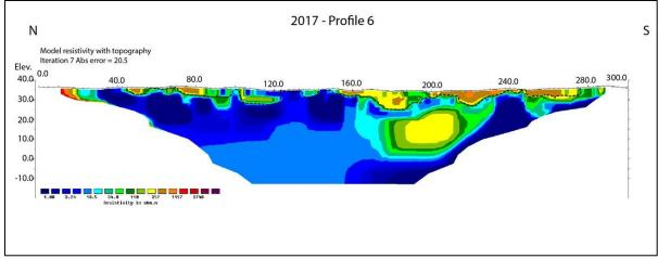
Figure 7.4: The Brenna area. The results from the 2D Resistivity measurements along profile 2017-6. The interpreted soil-bedrock interface is shown as a dotted black line.
