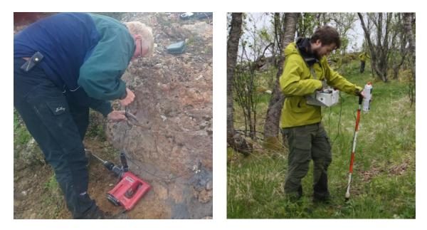
Figure 4.4: Establishing CP ore-grounding point (left) and data acquisition in combined CP and SP data (right).
