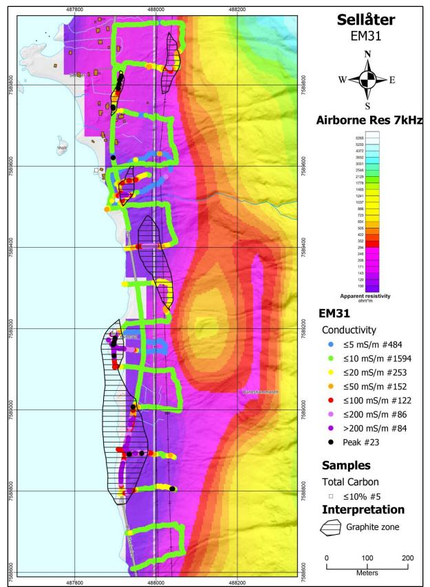
Figure 9.7: The Sellåter area. Interpreted graphite structures based on EM31 data, helicopterborne EM anomalies and exposures of graphite. The location of graphite samples and their Total Carbon content is given as white squares.
