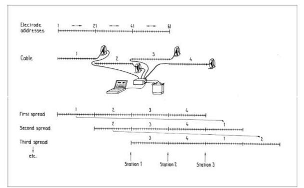
Figure 4.5: Diagram of measuring procedure illustrating the set-up of the Lund System and the roll-along method for performing as many measurements as required. (From ABEM 2012).
