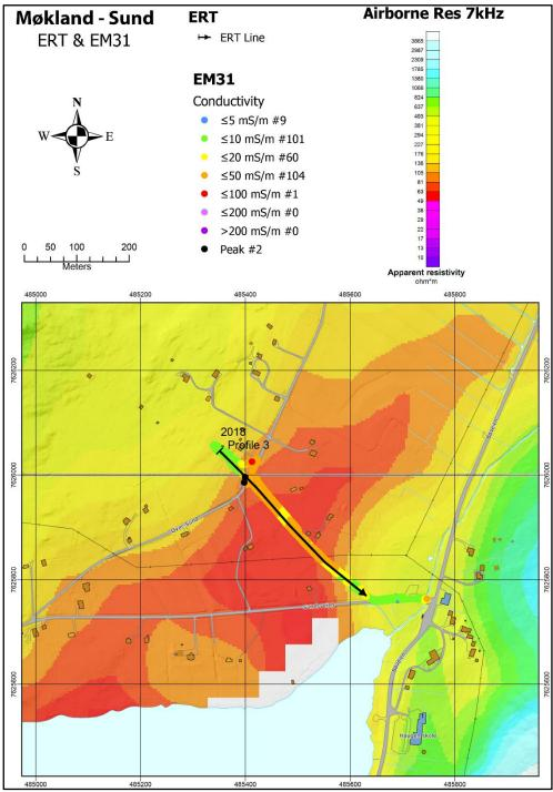
Figure 6.13: Results of EM31 measurements at Sund (southern part of Møkland area) superposed on apparent resistivity (7 kHz, from Rodionov et al. 2013a). Location of 2D ERT/IP profile is shown as a black line.
