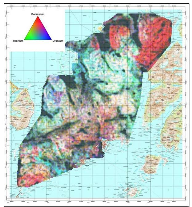
Figure 5.9: Radiometric ternary map (eU, eTh and K) from Austvågøya, Lofoten (from Rodionov et al. 2013b).
