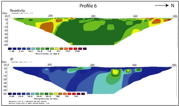
Figure 6.11: 2D resistivity (top) and IP (bottom) results along profile 2018-6 at Øyjorda. No graphite outcrops are observed.
