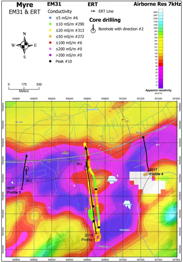
Figure 8.14: The area east of Myre. EM31 results and the location of 2D Resistivity/IP profiles are overlain helicopter-borne measurements of apparent resistivity from EM 7 kHz coaxial coil configuration (from Rodionov et al. 2013a). Location of ERT/IP profiles and drill-holes (Bh1 and Bh2) are indicated in black.
