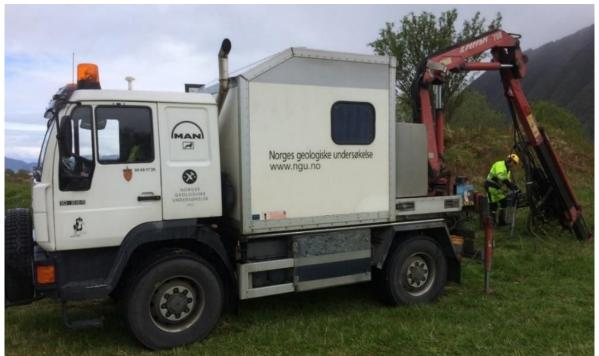
Figure 4.7: NGU's truck-mounted drilling gear in operation.
