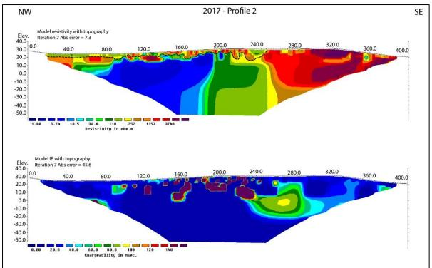
Figure 7.15: The Vikeid Central area. The results of the 2D Resistivity (ERT) and Induced Polarisation measurements along profile 2017-2. The interpreted soil-bedrock interface is marked as dotted black line.
