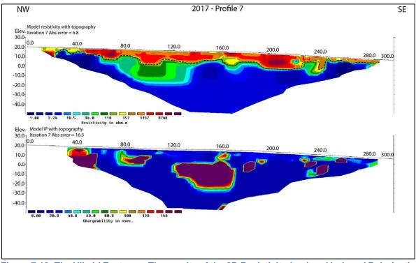
Figure 7.13: The Vikeid East area. The results of the 2D Resistivity (top) and Induced Polarisation (bottom) measurements along profile 2017-7. The interpreted soil-bedrock interface is marked as a dotted black line.
