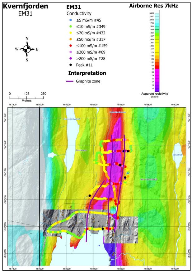
Figure 6.17: Kvernfjorden area. Interpreted near surface graphite structures based on helicopter-borne and ground-based EM geophysical data.
