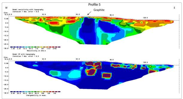
Figure 8.4: The Smines area. The results of the 2D Resistivity (ERT) and Induced Polarisation measurements along profile 2016-5.
