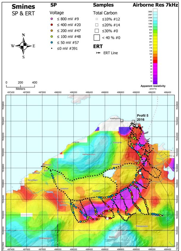
Figure 8.3: Results of SP measurements in the Smines area overlain on top of helicopter-borne measurements of apparent resistivity from EM 7 kHz coaxial coil configuration (from Rodionov et al. 2013a). The locations of graphite samples and their TC contents are shown as white squares, ERT/IP profile as black line.
