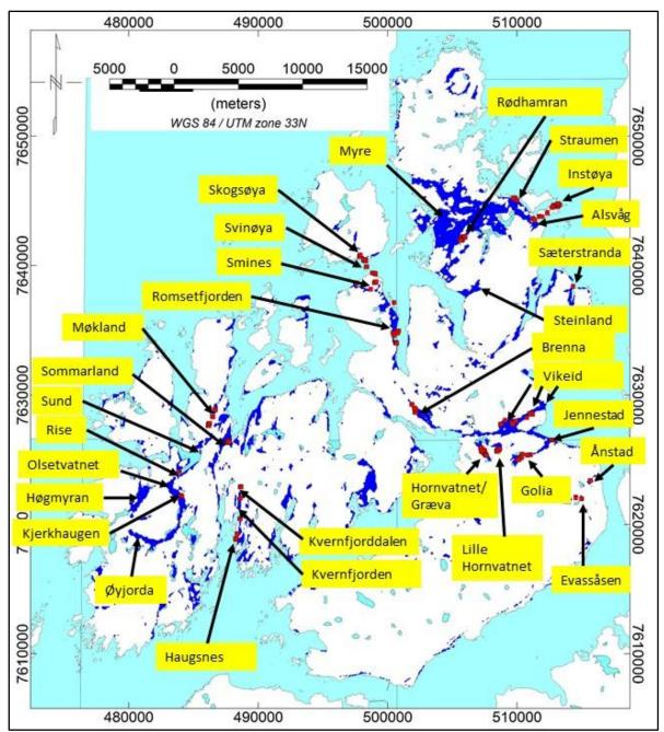
Figure 5.6: The blue colour shows areas on Langøya where apparent resistivity from EM 7 kHz coaxial coils is <300  $\Omega$ m and the magnetic anomaly field is <300 nT. The red squares show sample locations of graphite-bearing rock.
