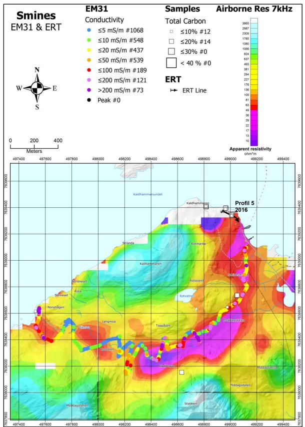
Figure 8.2: Results of EM31 measurements from the Smines area overlain helicopter-borne measurements of apparent resistivity from EM 7 kHz coaxial coil configuration (from Rodionov et al. 2013a). The locations of graphite samples and their TC contents are shown as white squares.
