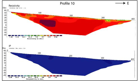
Figure 7.8: The Ånstad area. The results from the 2D Resistivity and IP measurements along profile 2019-2.
