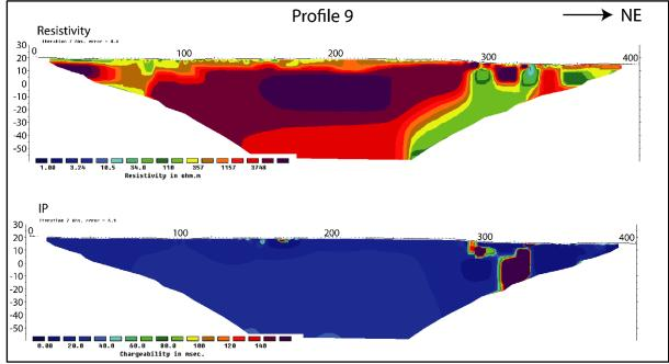
Figure 7.10: The Evassåsen area. The results from the 2D Resistivity and IP measurements along profile 2019-1.
