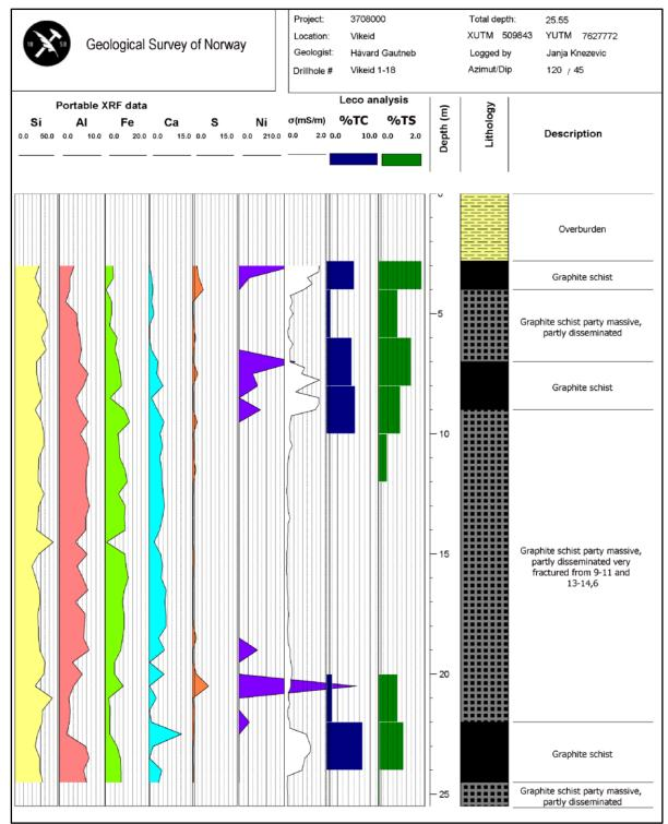
Figure 7.25: Results from the Vikeid Dh1-2018 drill-hole: Portable XRF analyses (Si, Al, Fe, Ca, and S in %, Ni in ppm) at the cores, downhole electric conductivity log ( $\sigma$ ), selected Leco analyses of Total Carbon (TC) and Total Sulphides (TS), lithological log and core description.
