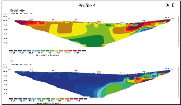
Figure 8.12: Steinland area. The results from 2D Resistivity and Induced Polarisation measurements along profile 2018-4.
