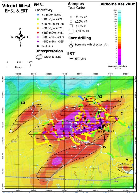
Figure 7.26: Interpreted graphite structures in the Vikeid West area. 3D inversion of helicopterborne EM data indicates that the Structures I, II, III and IV gives strong responses from ca. 10 m depth and down to 100 m and more. The Structure V shows up at only one resistivity level (36 – 54 m depth) while Structure VI seems to be a small surface phenomenon.
