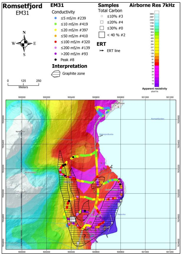
Figure 8.9: The area Romset in Romsetfjorden. Interpreted graphite structures (black line pattern) based on helicopter-borne EM, ground EM31 and graphite exposures. The location of graphite samples and their Total Carbon grade are shown as white squares.
