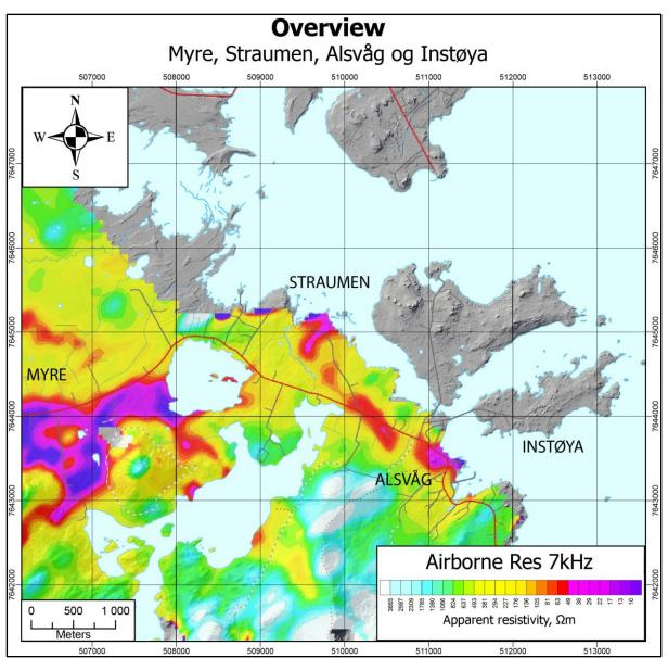
Figure 8.19: Alsvåg – Instøya – Straumen area. Apparent resistivity from helicopter-borne 7 kHz EM data (from Rodionov et al. 2013a). Instøya was not covered with helicopter-borne geophysics.
