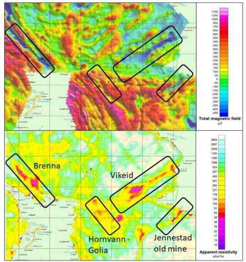
Figure 5.1: Magnetic anomaly field and apparent resistivity (7 kHz coaxial coils) from helicopterborne measurements in the Jennestad area, west of Sortland town (modified from Rodionov et al. 2013a).
