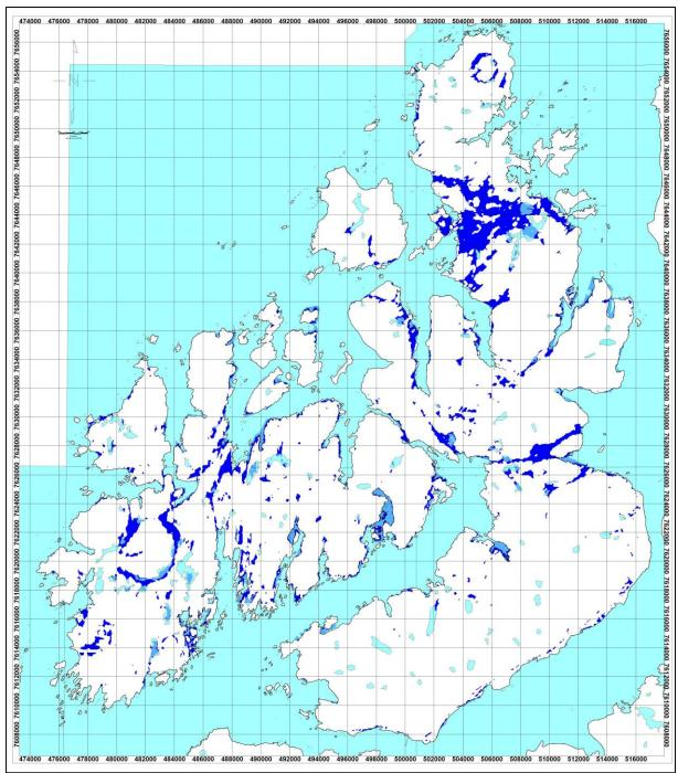
Figure 5.5: The blue colour shows areas on Langøya where apparent resistivity from EM 7 kHz coaxial coils is < 300  $\Omega$ m and magnetic total field is < IGRF + 300 nT.
