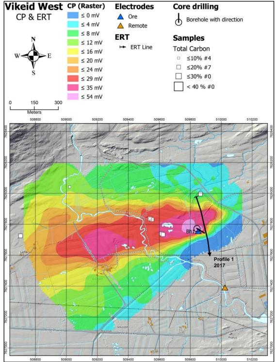
Figure 7.20: The Vikeid West area. Contour map of the CP data. Black lines show the location of ERT/IP profile. The locations of graphite samples and their TC contents are shown as white squares.
