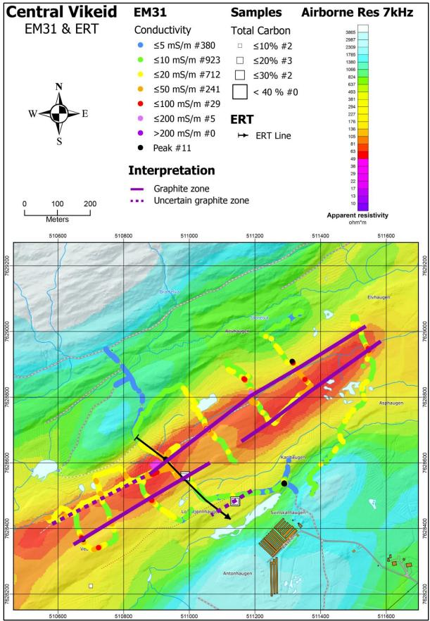
Figure 7.16: The Vikeid Central area. Interpreted graphite structures based on EM31 data, helicopter-borne EM anomalies and exposures of graphite. The locations of graphite samples and their TC contents are shown as white squares.
