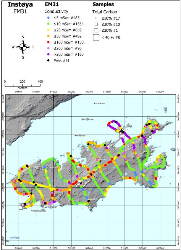
Figure 8.20: Instøya. Apparent conductivity values from EM31 measurements. The locations of graphite samples and their TC contents are shown as white squares.
