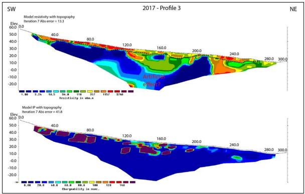
Figure 7.3: The Brenna area. The results from the 2D Resistivity and Induced Polarisation measurements along profile 2017-3. The interpreted soil-bedrock interface is shown as a dotted black line.
