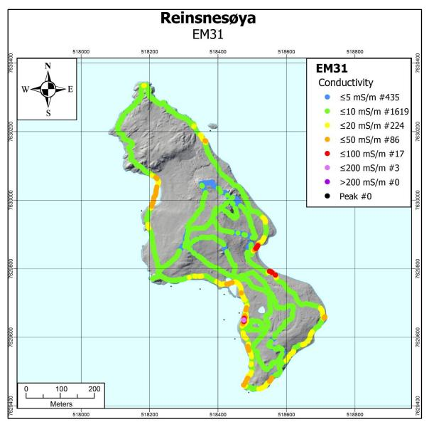
Figure 7.27: Results from EM31 measurements on the island Reinsnesøya.
