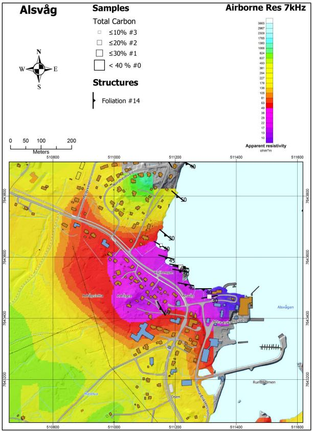
Figure 8.22: Alsvåg. Structural observations superposed on apparent resistivity from helicopterborne 7 kHz EM measurements (from Rodionov et al. 2013a). The locations of graphite samples and their TC contents are shown as white squares.
