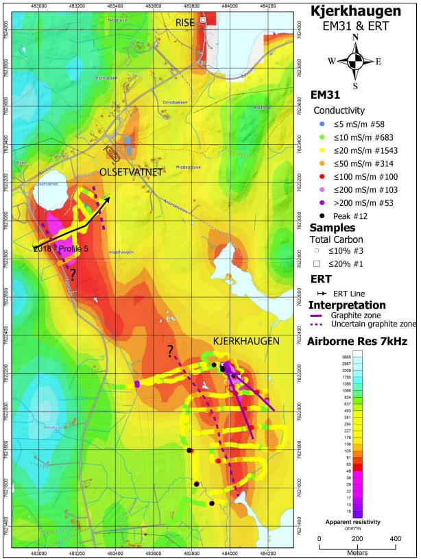
Figure 6.9: Rise, Olsetvatnet and Kjerkhaugen area. Interpreted near surface graphite structures based on ground and helicopter-based EM geophysical data and some exposures. Location of graphite samples and their TC content are shown as white squares.
