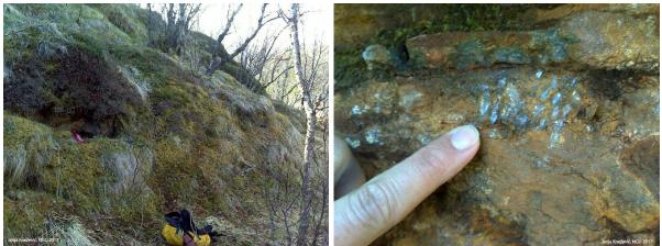
Figure 8.5: Graphite outcrop with 13.2 % TC and 0.33 % TS, sample JK-291517-9, UTM 499051 – 7638736.
