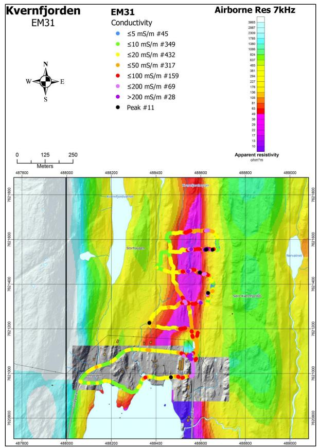
Figure 6.16: Results of EM31 measurements at Kvernfjorden superposed on apparent resistivity (7 kHz, from Rodionov et al. 2013a).
