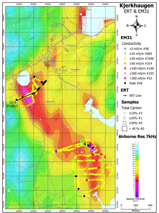
Figure 6.7: Results of EM31 measurements at Olsetvatnet and Kjerkhaugen superposed on apparent resistivity (7 kHz, from Rodionov et al. 2013a). Location of graphite samples and their Total Carbon grade is given as white squares. Location of 2D ERT/IP profile is shown as a black line.
