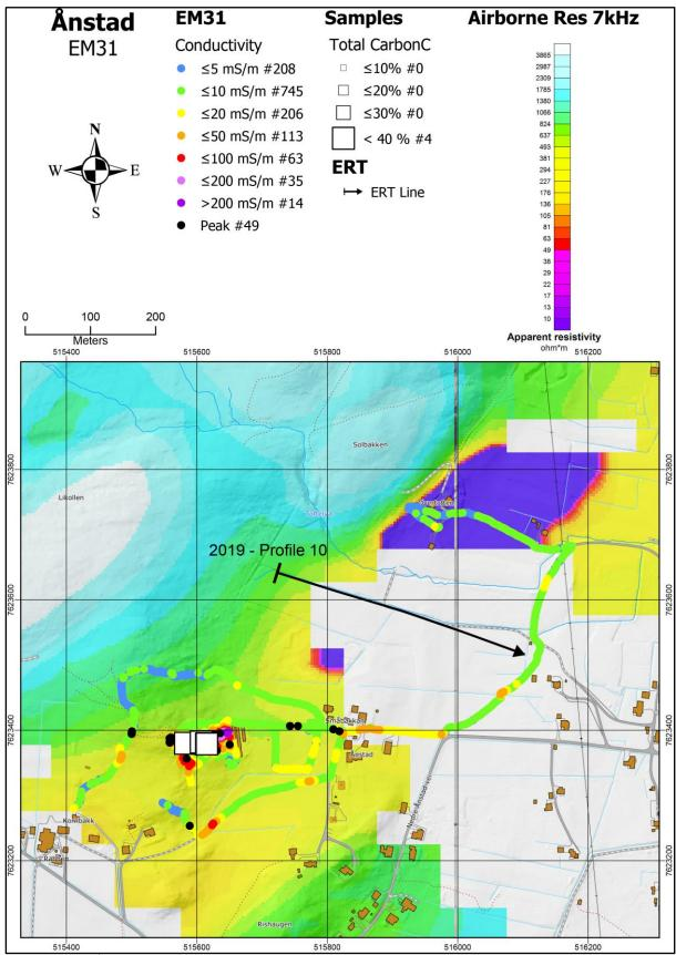
Figure 7.7: Ånstad. The results from the EM31 measurements superposed on apparent resistivity (EM 7 kHz coaxial coil configuration, Rodionov et al. 2013a). The locations of graphite samples and their TC content are shown as white squares, an ERT/IP profile as a black line.
