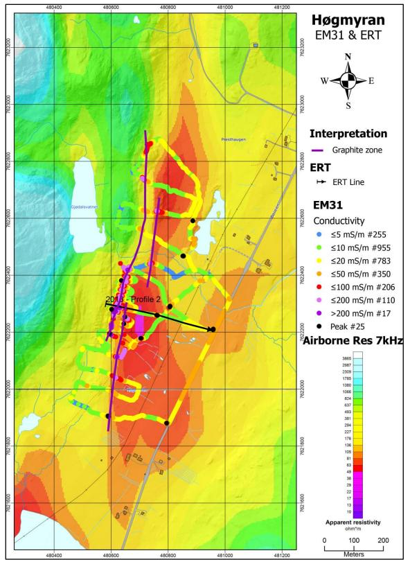
Figure 6.5: The Høgmyran area. Interpreted near-surface graphite structures based on ground and helicopter-borne EM geophysical data.
