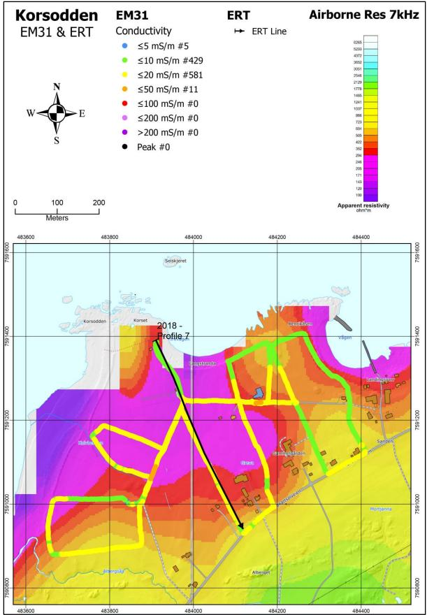
Figure 9.3: The Korsodden area. The results from the EM31 measurements superposed on apparent resistivity (EM 7 kHz coaxial coil configuration, Rodionov et al. 2013b).
