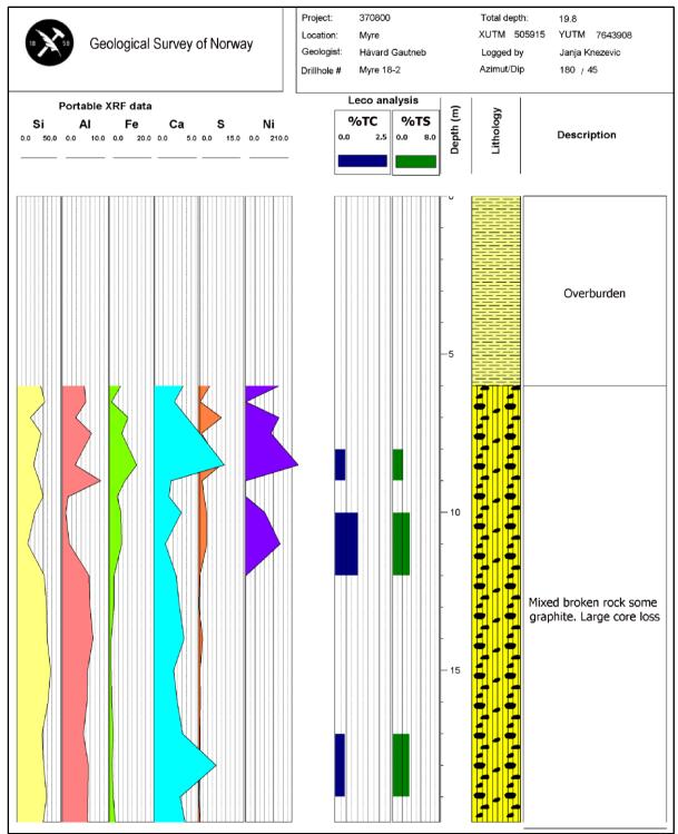
Figure 8.18: Results from the Myre drill-hole Dh2-2018: Portable XRF analyses (Si, Al, Fe, Ca, and S in %, Ni in ppm) at the cores, selected Leco analyses of Total Carbon (TC) and Total Sulphides (TS), lithological log and core description.
