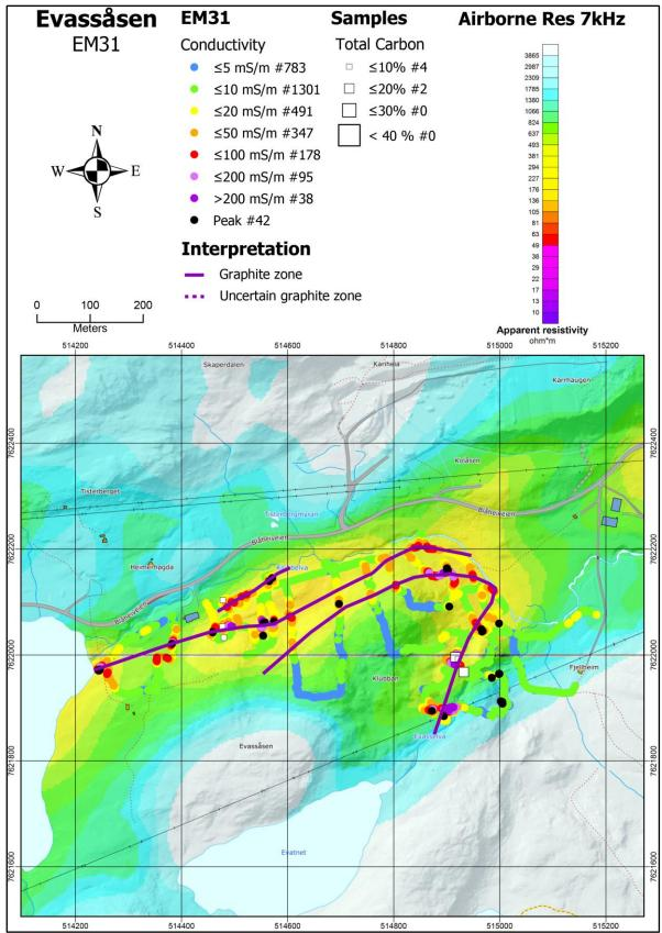
Figure 7.11: Evassåsen interpretation map. The results from the EM31 measurements are superposed on apparent resistivity (EM 7 kHz coaxial coil configuration, Rodionov et al. 2013a) and interpreted graphite mineralisation. Sample locations and TC contents are shown as white squares. Interpreted graphite structures are shown as violet lines.
