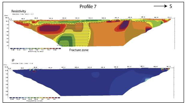
Figure 9.4: The Korsodden area. The results of the 2D Resistivity and Induced Polarisation measurements along profile 2018-7. The interpreted soil-bedrock interface is presented as a dotted black line and a possible fractured zone in bedrock as horizontal line pattern.
