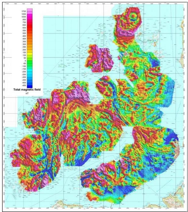
Figure 5.3: Magnetic anomaly field on Langøya, Vesterålen (from Rodionov et al. 2013a).
