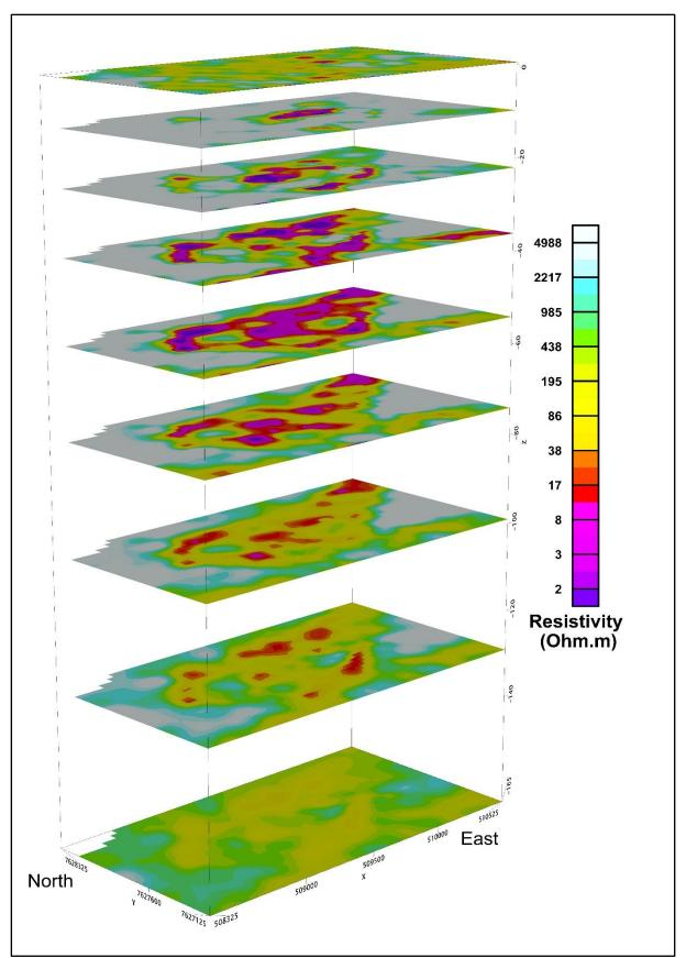
Figure 7.24: The results from 3D inversion of helicopter-borne EM data. Resistivity distributions in individual levels are plotted on top of the levels and represent the resistivity values down to the next level.
