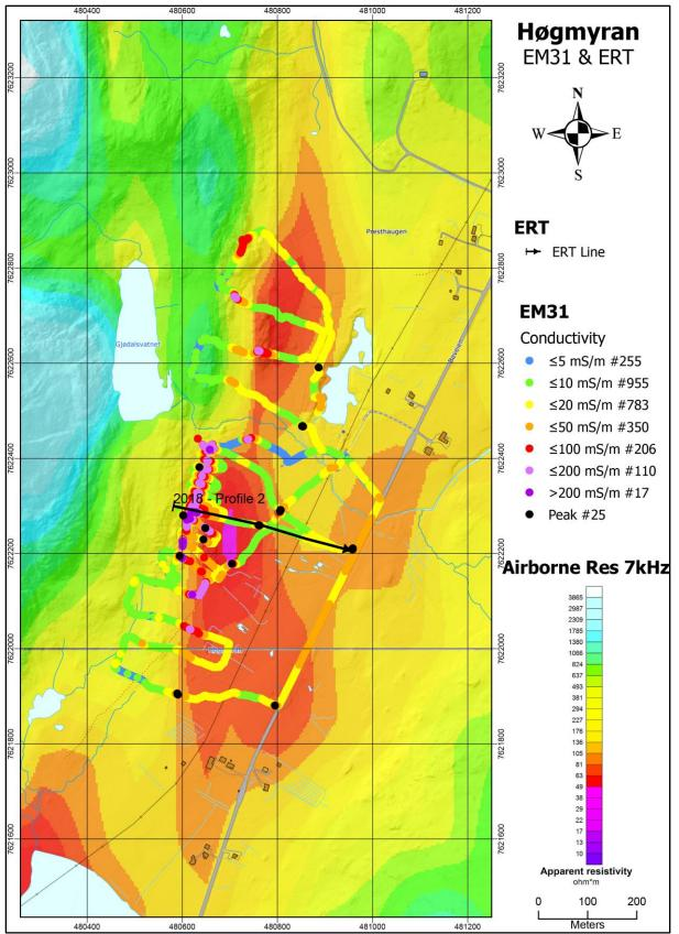
Figure 6.3: Results of EM31 measurements at Høgmyran superposed on apparent resistivity (7 kHz, from Rodionov et al. 2013a). Location of 2D ERT/IP profile is shown as a black line.
