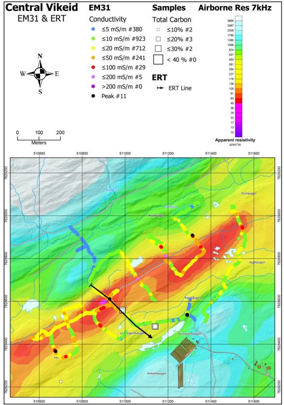
Figure 7.14: The Vikeid Central area. The results from the EM31 measurements are superposed on apparent resistivity (EM 7 kHz coaxial coil configuration, Rodionov et al. 2013a). Black lines show the location of the ERT/IP profile. The locations of graphite samples and their TC content are shown as white squares.
