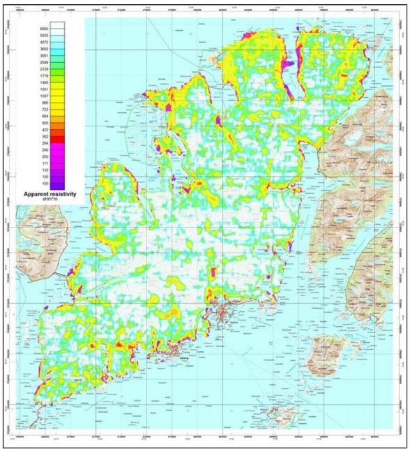
Figure 5.7: Apparent resistivity calculated from EM 7 kHz Coaxial coil configuration on parts of Austvågøya, Lofoten (from Rodionov et al. 2013b).
