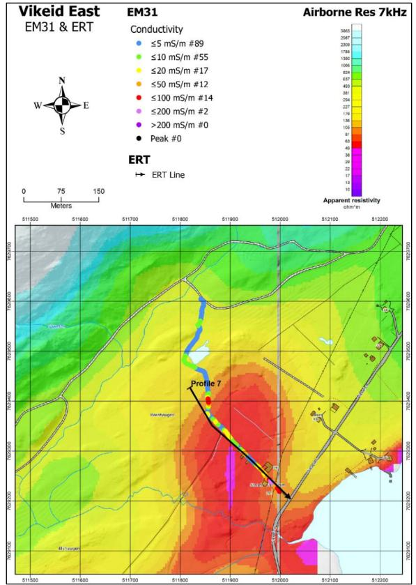
Figure 7.12: The Vikeid East area (Storelvbukta). The results from the EM31 measurements are superposed on apparent resistivity (EM 7 kHz coaxial coil configuration, Rodionov et al. 2013a). Black lines show the location and direction of the ERT/IP profiles.
