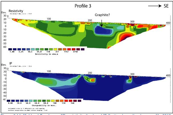
Figure 6.14: Møkland-Sund area. 2D resistivity (top) and IP (bottom) results along profile 2018-3. No graphite outcrops are observed.
