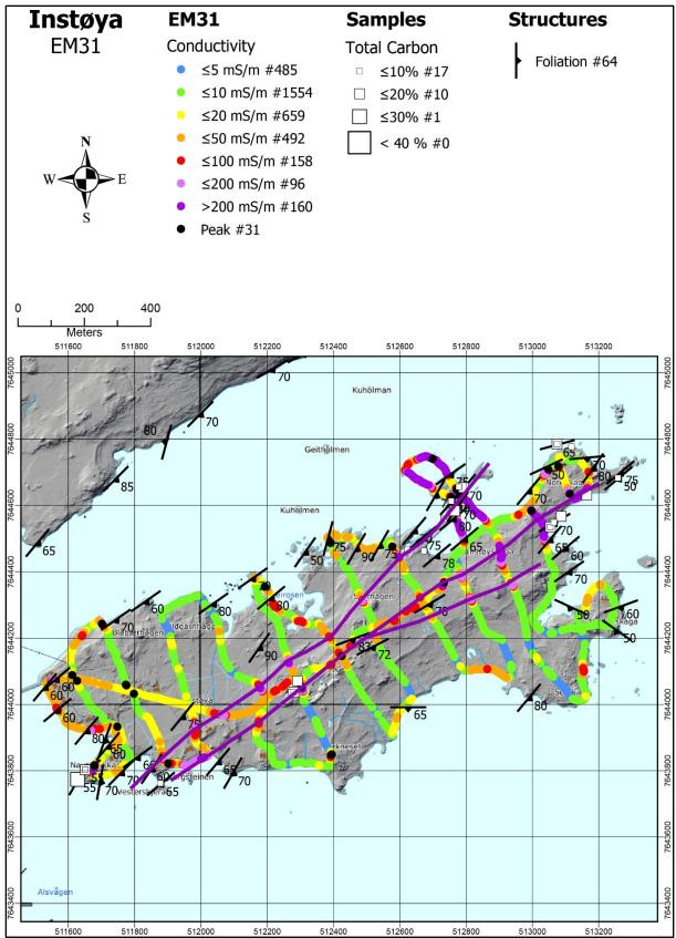
Figure 8.21: Instøya. Interpreted graphite structures (purple lines) from EM31 data and strike/dip observations. The locations of graphite samples and their TC contents are shown as white squares.
