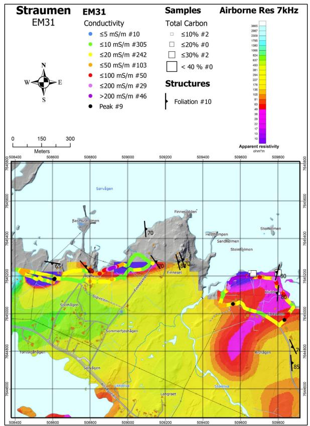
Figure 8.23: Straumen. Strike and dip observations and apparent electric conductivity from EM31 measurements superposed on apparent resistivity from 7000 Hz helicopter-borne EM (from Rodionov et al. 2013a). The locations of graphite samples and their TC contents are shown as white squares.
