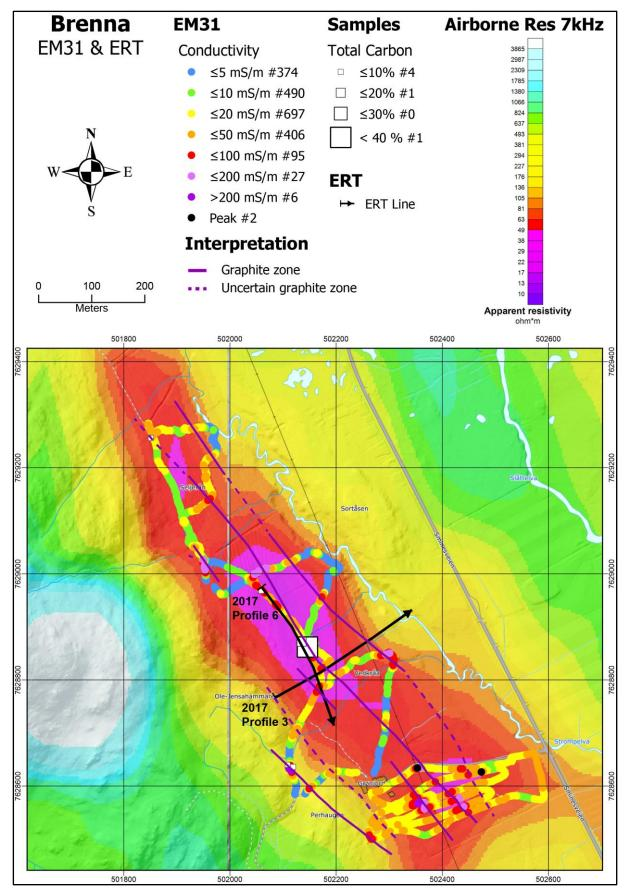
Figure 7.5: The Brenna area. The interpreted near-surface graphite structures are based on exposures, EM31 and helicopter-borne EM data. The locations of graphite samples and their TC content are shown as white squares.
