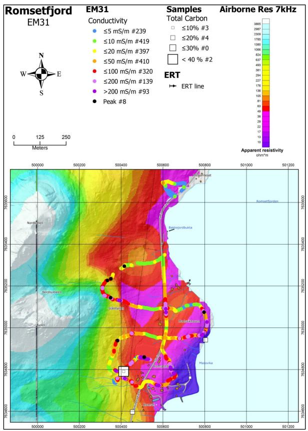
Figure 8.7: Results of EM31 measurements from the Romset area in Romsetfjorden, overlain helicopter-borne apparent resistivity from EM 7 kHz coaxial coil configuration (from Rodionov et al. 2013a). The location of graphite samples and their Total Carbon grade are shown as white squares.
