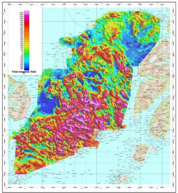
Figure 5.8: Magnetic anomaly field in parts of Austvågøya, Lofoten (from Rodionov et al. 2013b).
