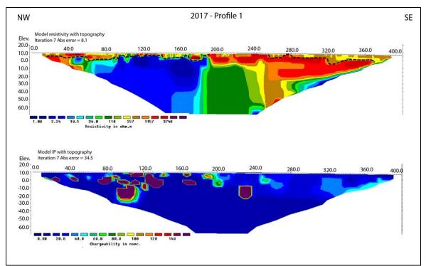
Figure 7.19: The Vikeid West area. The results of the 2D Resistivity (ERT) and Induced Polarisation measurements along profile 2017-1. The interpreted soil-bedrock interface is indicated as the dotted black line.
