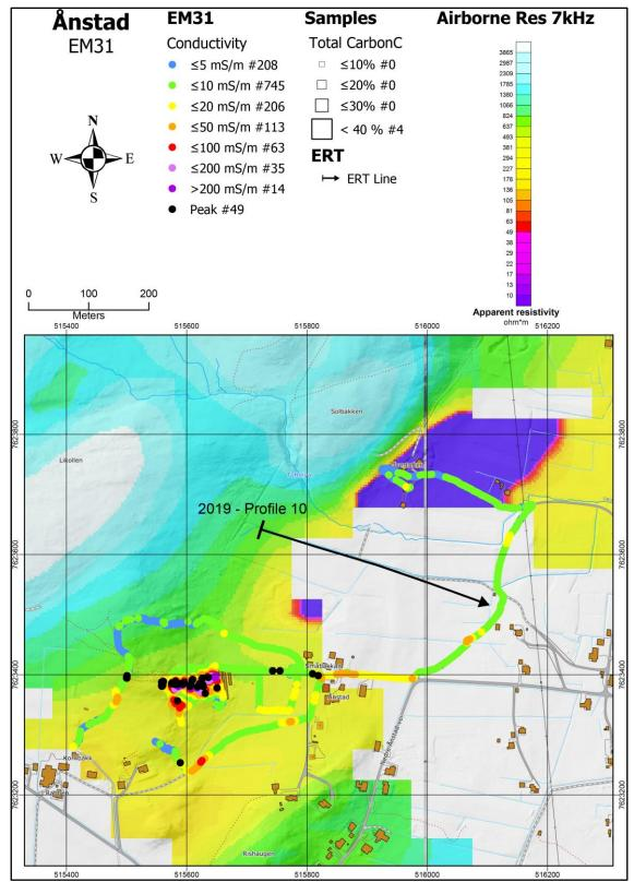
Figure 7.6: Ånstad. The results from the EM31 measurements superposed on apparent resistivity data (EM 7 kHz coaxial coil configuration, Rodionov et al. 2013a). The ERT/IP profile measured in 2019 is shown as a black line.
