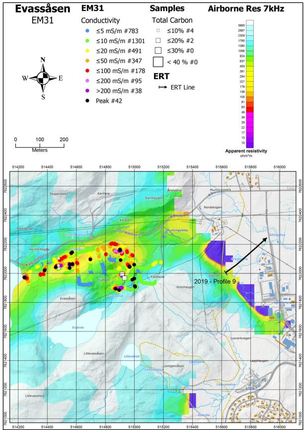
Figure 7.9: Evassåsen. The results from the EM31 measurements superposed on apparent resistivity (EM 7 kHz coaxial coil configuration, Rodionov et al. 2013a). Locations of graphite samples and their TC content are shown as white squares and the ERT/IP profile as a black line.
