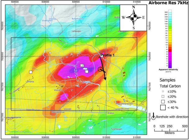
Figure 7.23: The Vikeid West area: Area for 3D inversion of helicopter-borne EM data (black rectangle). The ERT/IP profile is marked as a black line.
