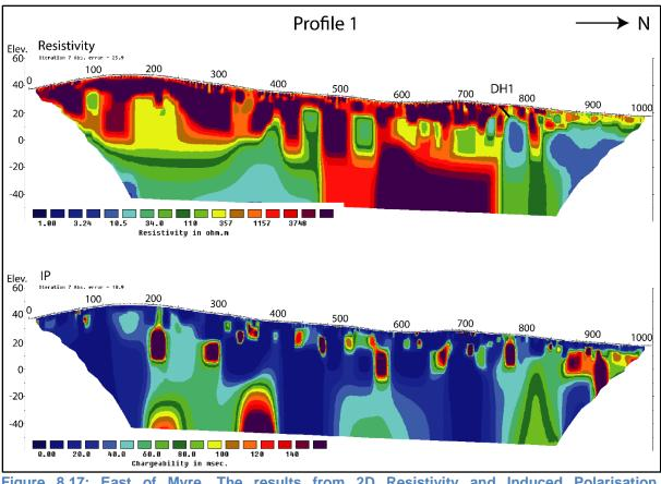
Figure 8.17: East of Myre. The results from 2D Resistivity and Induced Polarisation measurements along profile 2018-1. The soil-bedrock interface is not easy to see in this profile except for the northern part where a soil thickness of 5 to 10 metres is indicated. Drill-hole Dh1 is indicated as a black line.
