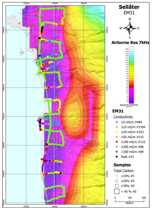
Figure 9.6: The Sellåter area. The results from the EM31 measurements superposed on apparent resistivity (EM 7 kHz coaxial coil configuration, Rodionov et al. 2013b). The location of graphite samples and their Total Carbon content is given as white squares.
