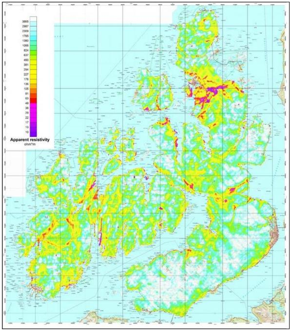
Figure 5.2: Apparent resistivity calculated from EM 7 kHz Coaxial coil configuration at Langøya in Vesterålen (from Rodionov et al. 2013a).
