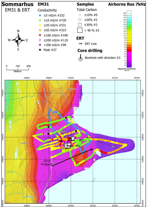
Figure 9.9: The Sommarhus area. The results from the EM31 measurements superposed on apparent resistivity (EM 7 kHz coaxial coil configuration, Rodionov et al. 2013b). The location of graphite samples and their Total Carbon content is given as white squares.
