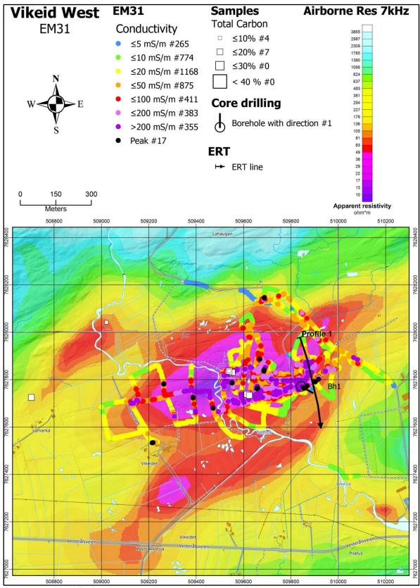
Figure 7.18: The Vikeid West area. The results from the EM31 measurements are superposed on apparent resistivity (EM 7 kHz coaxial coil configuration, Rodionov et al. 2013a). Locations of graphite samples and their TC contents are shown as white squares.
