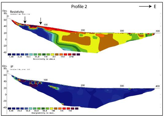
Figure 6.4: 2D resistivity (top) and IP (bottom) results along profile 2018-2 at Høgmyran. No graphite outcrops are observed. Potential (interpreted) graphite zones are indicated with black arrows.
