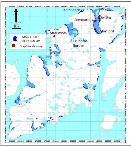
Figure 5.10: The blue colours shows areas on Austvågøya where apparent resistivity from EM 7 kHz coaxial coils is < 300  $\Omega$ m and magnetic total field is < IGRF 2015 + 300 nT. The red squares are samples of graphite-bearing rock.
