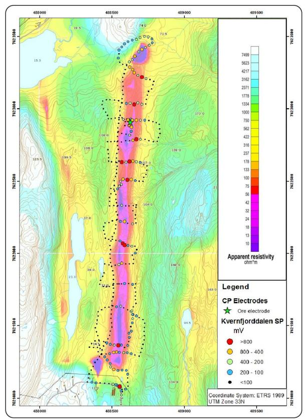
Figure 6.15: Kvernfjorddalen. SP anomalies superposed on airborne apparent resistivity calculated from 6600 Hz coplanar coils (from Rønning et al. 2017).
