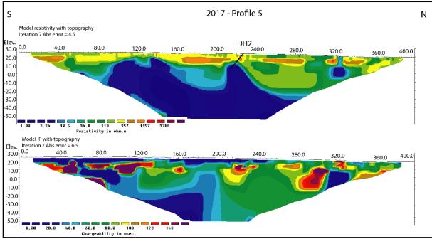
Figure 8.16: The area east of Myre. The results from 2D Resistivity and Induced Polarisation measurements along profile 2017-5. Drill-hole Dh2 is shown as a black line.
