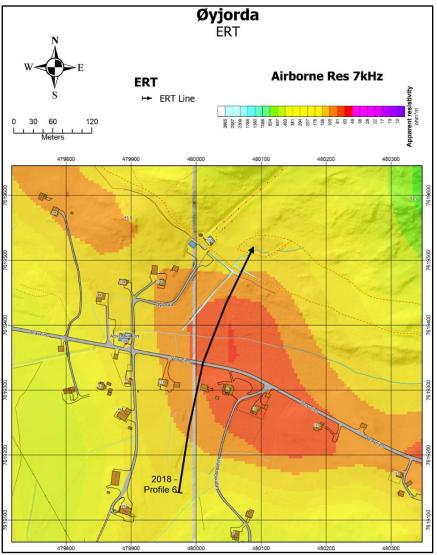
Figure 6.10: The location of the ERT/IP profile at Øyjorda superposed on apparent resistivity (7 kHz, from Rodionov et al. 2013a).
