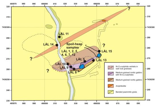
**Figure 50.** Geological map of the Lilleålegden mining area showing the locations at which samples were collected.
