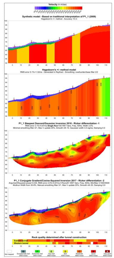
Figure 7.1.1: P1\_1 comparison between old and new inversion result. From top to bottom: Traditional interpretation (Wåle, 2009) - 2D Plus-Minus method model as constructed in Rayfract<sup>®</sup> - Result using Single-run Steepest Descent/Gaussian inversion (Rønning et al., 2016) - Result using the Multi-run Conjugate
