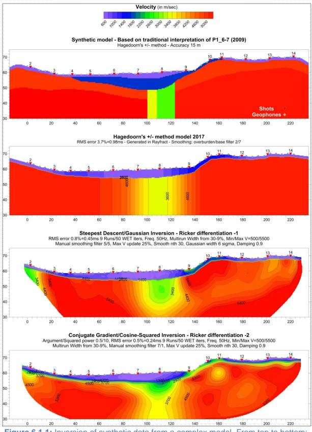
Figure 6.1.1: Inversion of synthetic data from a complex model. From top to bottom: synthetic model based on Profile P1\_6-7 from Knappe - 2D Plus-Minus method model as constructed in Rayfract<sup>®</sup> - Inversion result using the Steepest Descent/Gaussian inversion scheme - Inversion result using the Conjugate Gradient/Cosine-Squared inversion scheme.
