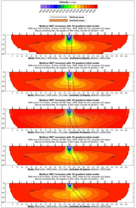
**Figure 5.4.1:** Effect of fracture zone inclination in **multi-run WET inversion** using Conjugate Gradient method and **Gaussian weighting** (from top 0°, 15°, 30°, 45° and 60° from vertical).
