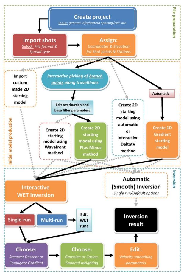
Figure 2.1: Flowchart for Rayfract® software. Black arrows shows procedures we have used, gray dotted arrows other options available with the software.
