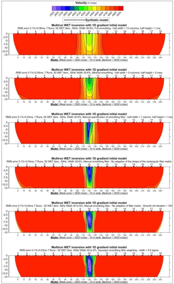
**Figure 4.5:** Simple fracture zone in bedrock: 7 step multi-run WET inversion using variable wavepath width 30 – 6 % and decreasing smoothing.
