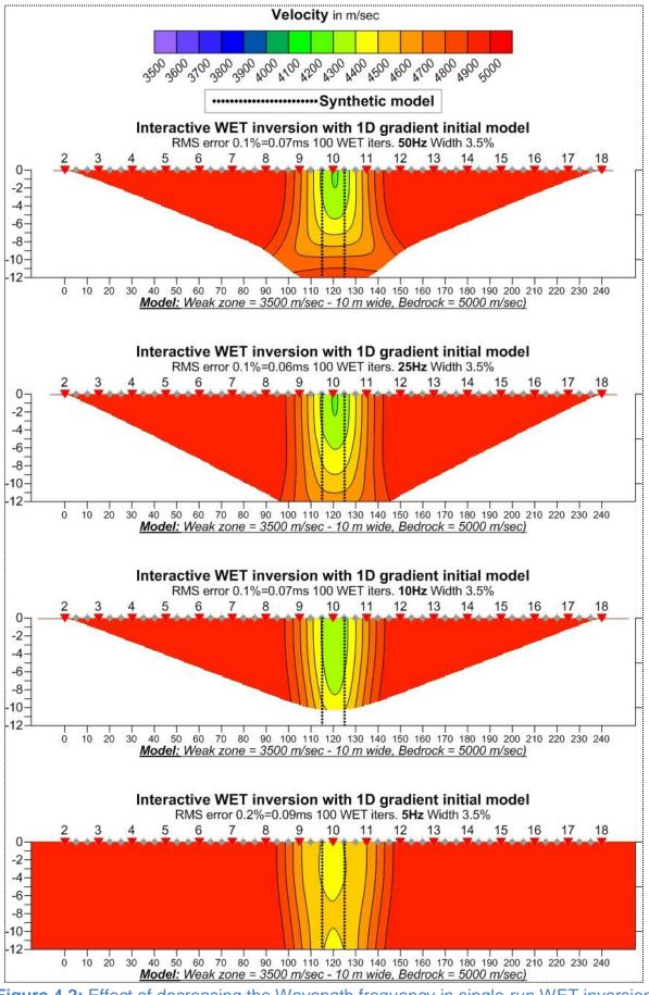
Figure 4.2: Effect of decreasing the Wavepath frequency in single-run WET inversion (from top 50, 25, 10 and 5 Hz).
