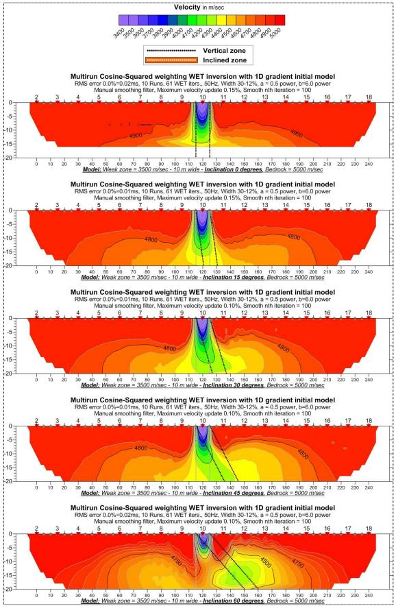
**Figure 5.4.2:** Effect of fracture zone inclination in **multi-run WET inversion** using Conjugate Gradient method and **Cosine-Squared weighting** (from top 0°, 15°, 30°, 45° and 60° from vertical).
