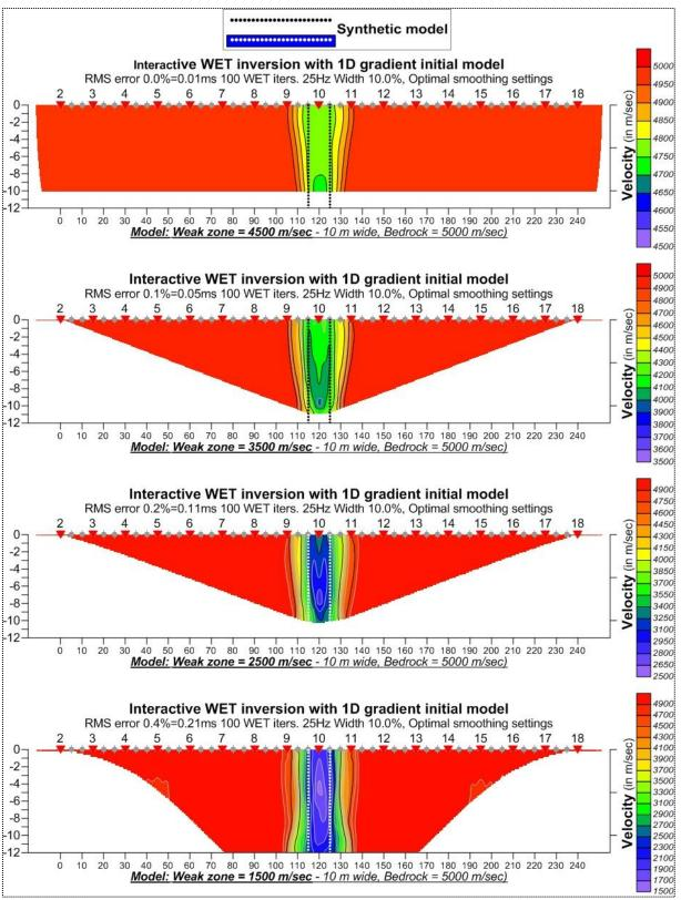
Figure 5.1.1: Effect of velocity contrast between fracture zone and bedrock in singlerun WET inversion (weak zone: from top 4500, 3500, 2500 and 1500 m/s).
