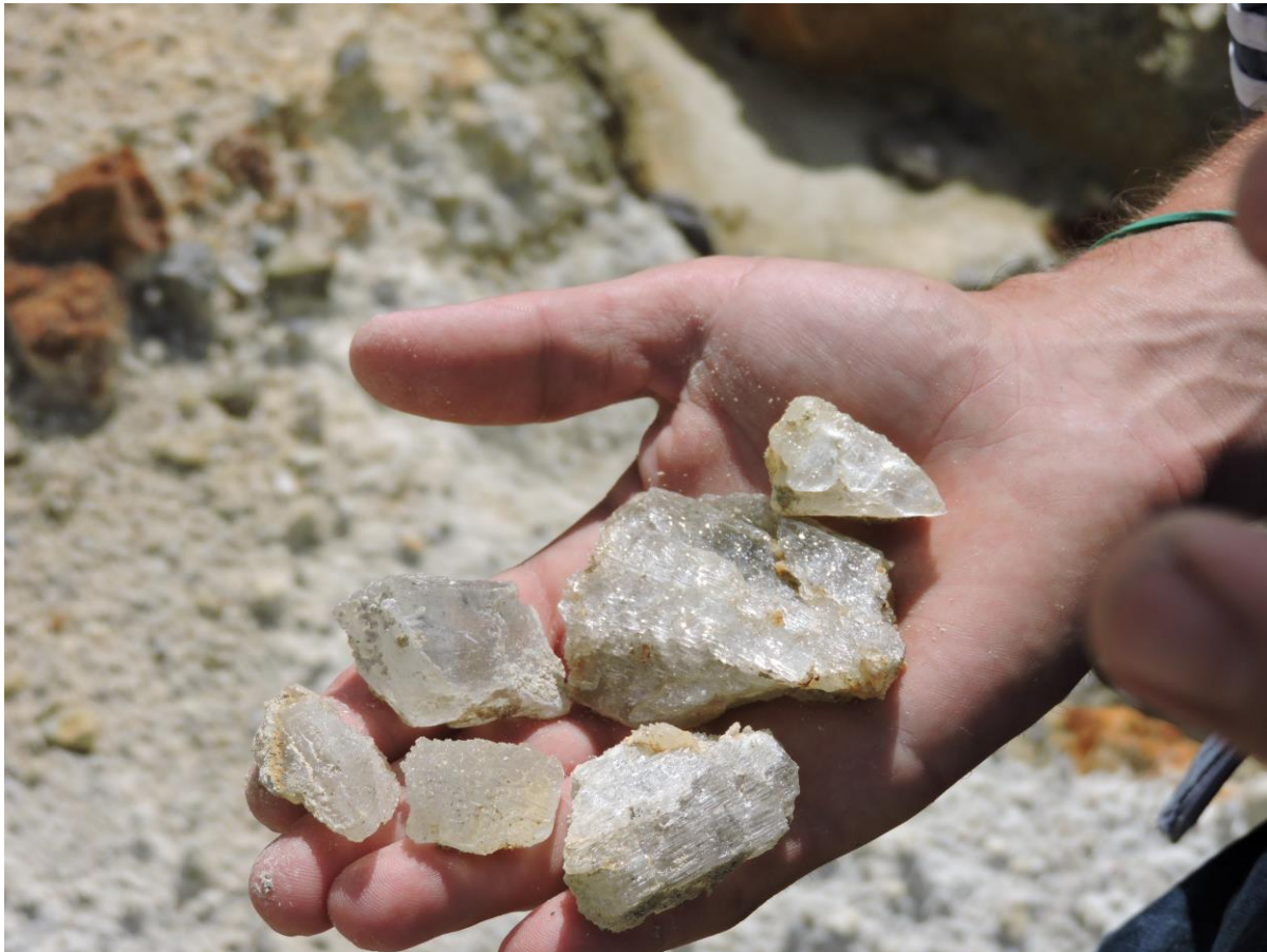
Figure 6.6. Gypsum mineralisation found within tailings material at Balei. (Photo by Dave Banks).
