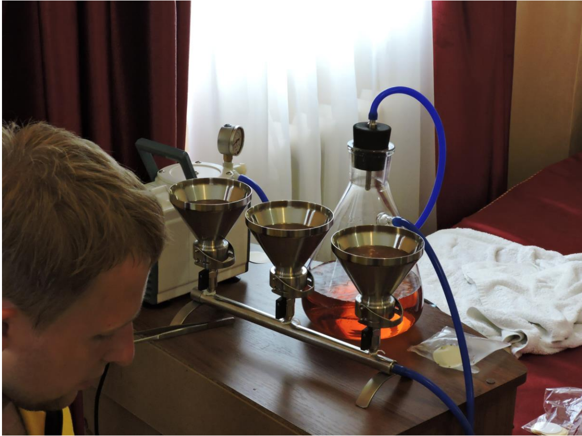
Figure 3.8 (above). Filtering mine water samples to obtain microbiological samples (Photo by David Banks).
