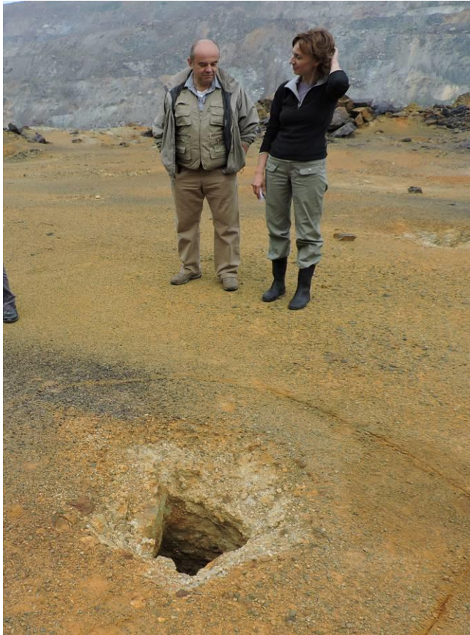
Figure 3.7. Borehole in bench of the polymetallic opencast at Sherlovaya Gora (Photo by David Banks)
