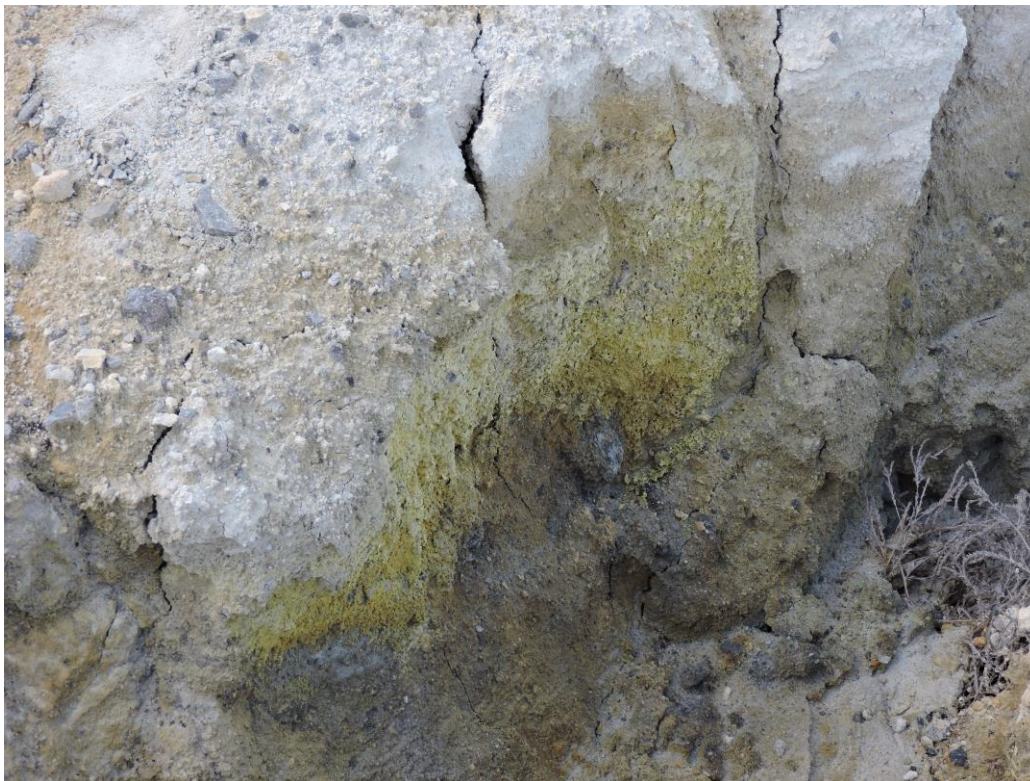
Figure 6.5. Presumed jarosite mineralisation with tailings area embankment at Balei. (Photo by Dave Banks).
