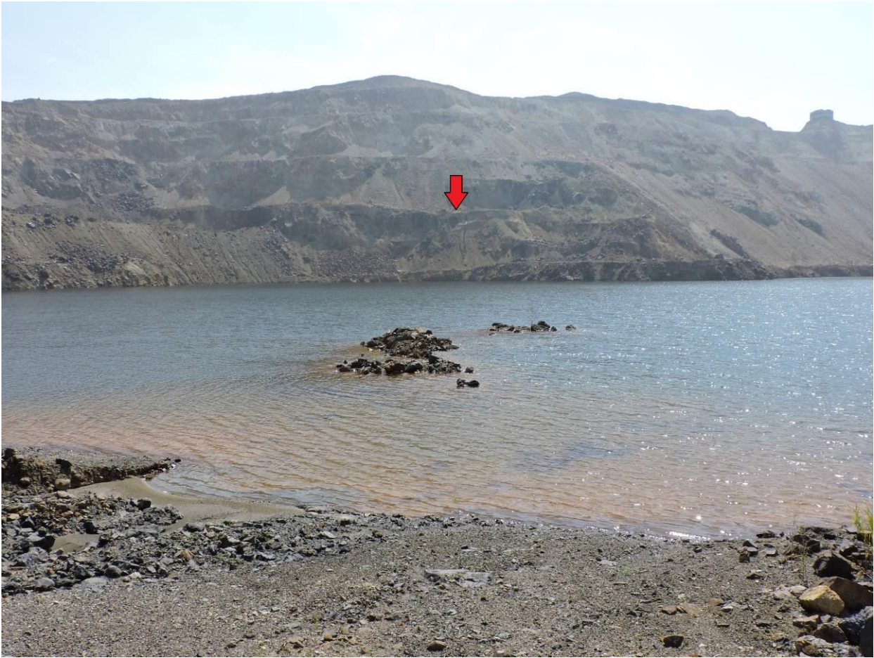
Figure 3.10. The polymetallic opencast at Sherlovaya Gora, seen from sampling point for Shg-101, looking east. The red arrow indicates the bench into which the sampled boreholes were drilled. Note the iron oxyhydroxide staining of the lake bed near the shore (Photo by David Banks)
