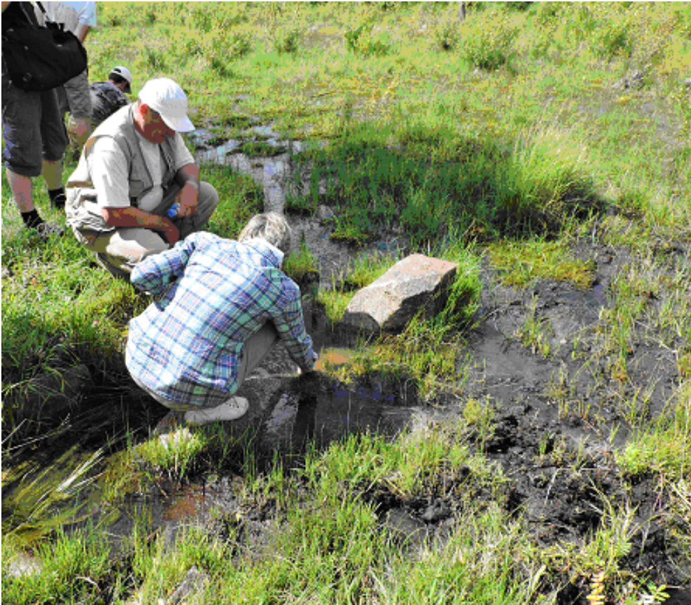
Figure 4.7. Spring at eastern end of foot of dam at base of lower tailings level at Novii Akatui (pH 6.7, +258 mV, samples Shg-04F). (Photo by David Banks)
