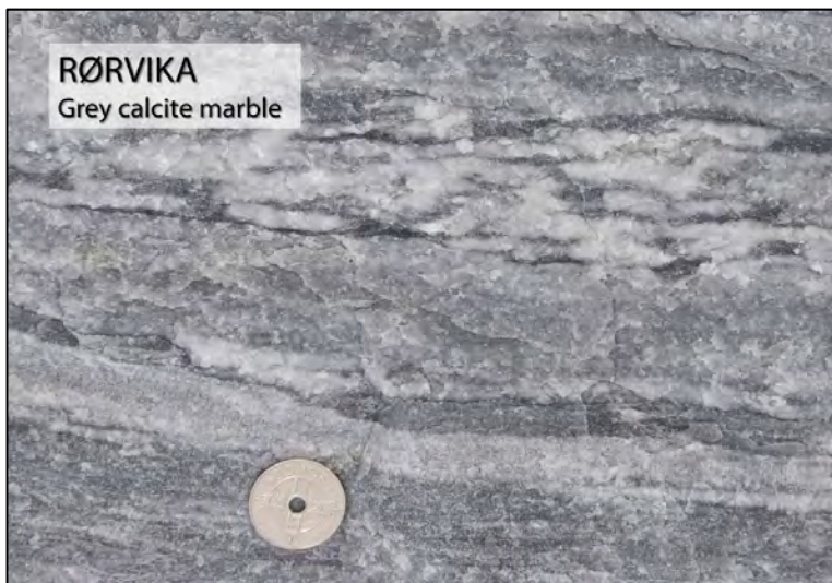
Fig. 4: Close-up photo of a heterogeneous, strongly deformed, grey calcite marble from Rørvika, Evenes, Nordland.
