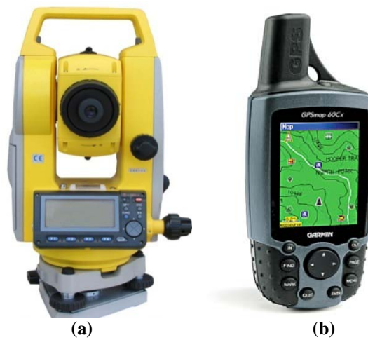
Figure 2.2 Leveling instruments: (a) Total station survey camera for height measurements, (b) GPSMap 60Cx used for horizontal location of the gravity points.
