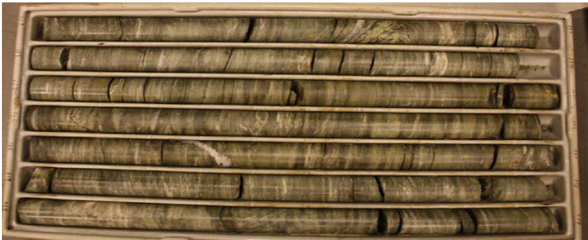
Figure C- 1. Picture of the well foliated quartz-rich greenstones that are typical of the 95 – 123 m core interval with epidote-rich bands and epidote-bearing fold hinges (one can be seen at the top of the picture). (Core interval of the box: 112 – 119 m from the top left to the bottom right).
