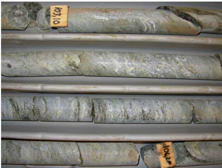
Figure C- 5. Picture of the very quartz-rich folded and well foliated greenstones and schists of the 96 – 120 m drill core interval. Note the fold hinge at the top of the picture. The green veins are epidote-filled.
