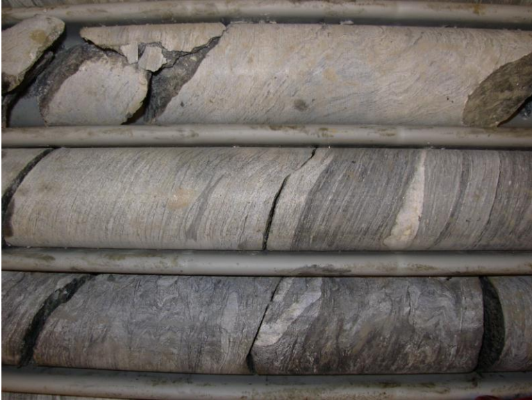
Figure B- 19. Sharp boundary between two compositions of black shales at 794 m along the core, i.e. between the graphite-rich (dark) layers of the 496.3 – 794 m core interval and the graphite-poor (pale gray) layers of the 794 – 850 m core interval.
