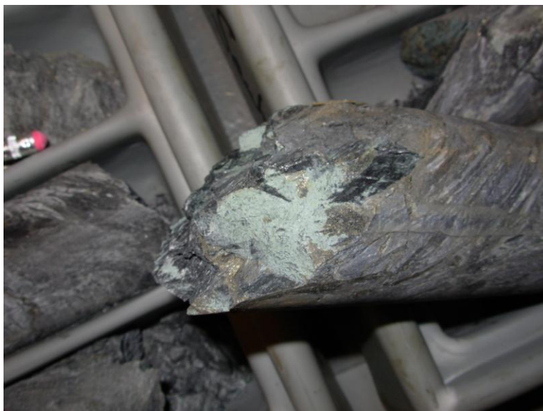
Figure B- 14. A typical pyrite and green Cu-rich coating of fracture surface in the black shales at 595 m along the core.
