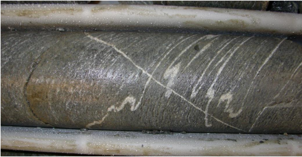
Figure B- 15. A typical ptygmatic fold of quartz layer in the black shale at 608.7 m along the core.
