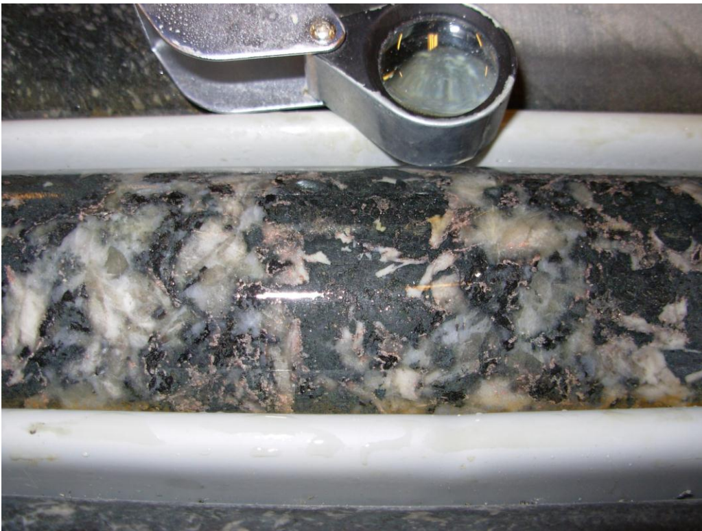
Figure A- 3. A 10 cm thick very coarse-grained gabbro with pink garnet rims around biotites (?) in the 79 – 87 m core interval.
