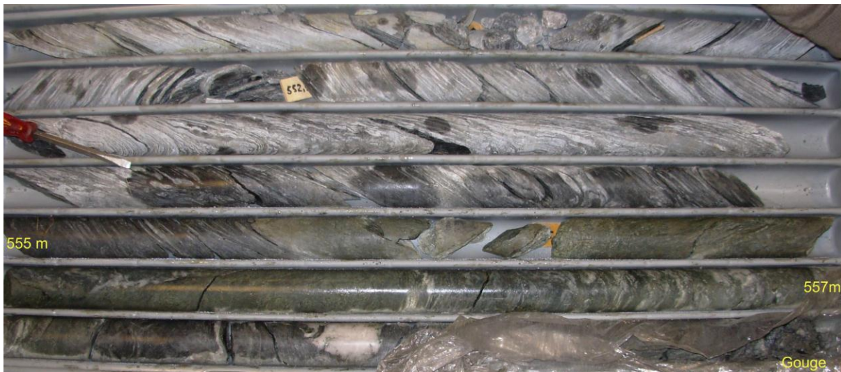
Figure B- 11. Green (chloritization?) alteration of the black shales in the 555.5 – 557 m core interval and clays/ fault gouge of the 557.6 – 558 m core interval.
