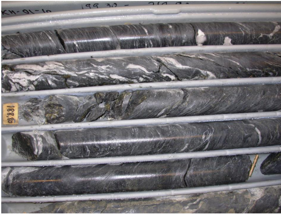
Figure B- 5. Typical facies of the black shales with sheared/eye-shaped quartz patches.
