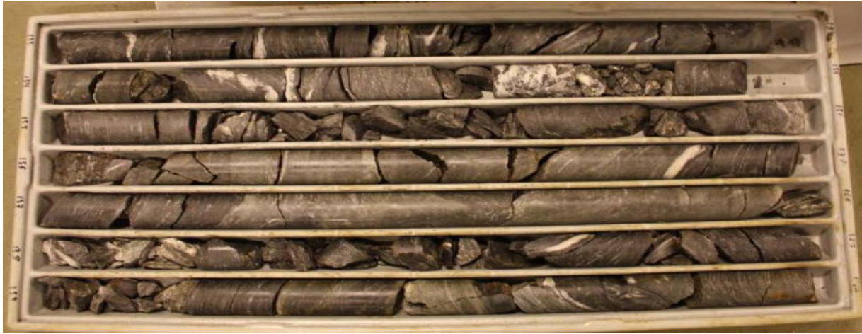
Figure C- 2. Picture of the folded and foliated black shales with crushed rocks here in the 133 – 140 m core interval. They are typical of the entire 131 – 148 m core interval.
