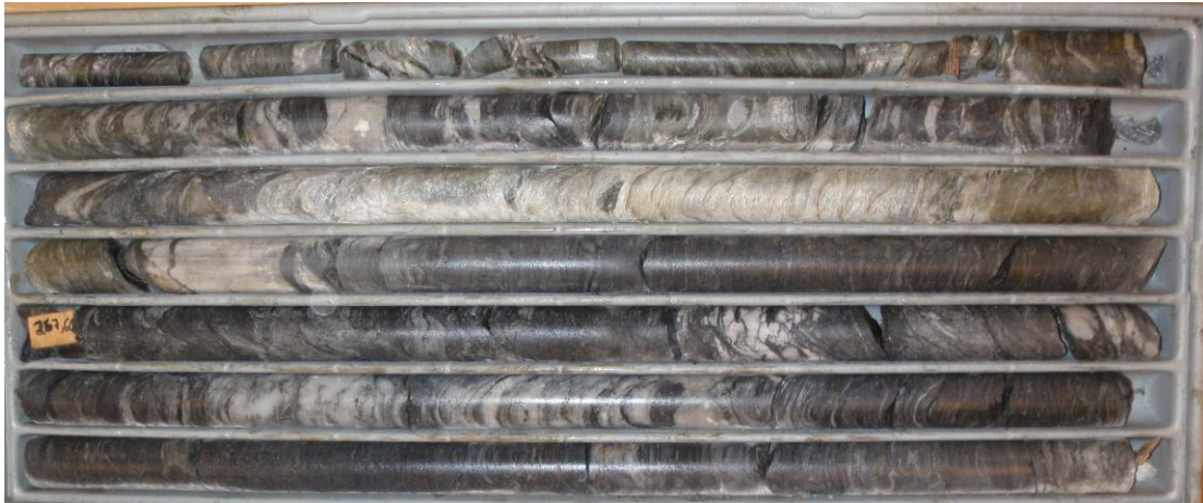
Figure C- 4. Picture of the core interval 233.8 – 240.4 m (from top left to bottom right in the box) that illustrates the foliated and folded greenstones with some graphite-rich and quartz-rich schist layers of the 203 – 249.4 m interval with, at the bottom of the picture, the foliated and sheared quartz-rich schists of the 236.7 – 249.4 m sub-interval.
