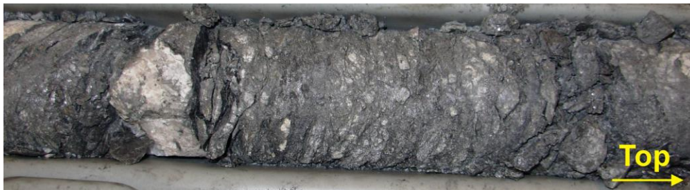
Figure C- 8. At c. 287 m, example of the clay-rich silty to sandy grain size breccia with fragmented quartz in the large fault rock zone of the 275– 295 m core interval.
