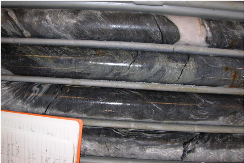
Figure B- 20. Folded chlorite-rich layer at 878 m and other typical folds of the surrounding black shales.
