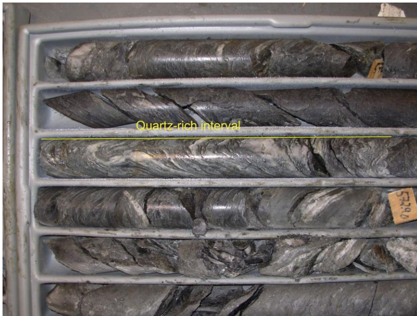
Figure B- 12. Quartz-rich schist inter-layered within the graphite-rich black shales at c. 571.5 m along the core.
