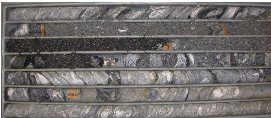
Figure 6. Silty to sandy grain size breccias in the graphite-rich black shale layer of the 665.8 – 668 m core interval.
