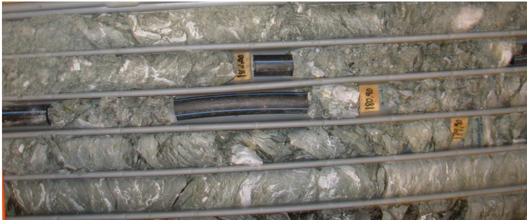
Figure B- 3. The quality of the rocks is very poor between c. 179 m and 183 m with numerous crushed zones, i.e. breccias, and the presence of a soapy mineral (talc?). Note the presence of fragmented/brecciated angular quartz grains that testifies to fault rock formation.
