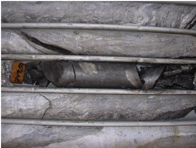
Figure B- 18. Graphite-rich layer at 749.5 m along the core in a quartz- and muscovite-rich black shale interval.
