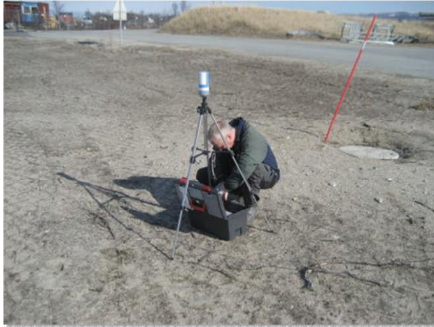
Figure 2.4 Geir Viken next to the base station magnetometer deployed in Lakselv during the BASAR-08 acquisition.
