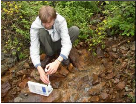
Figure 10.9. DB titrates alkalinity at Starii Berikul' adit (Xa113)
