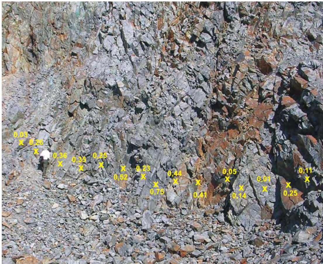
Figure 9: Cu-analyses (in %) by handheld XRF-analyzer along a profile in the lowermost NE-wall in 'Hovedfelt' (for location see Figure 2).
