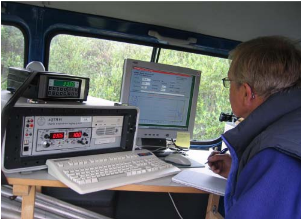
Figure B3. The electronic unit. Measured temperatures together with other recorded parameters (depth, weight of probe and cable and logging speed) can be followed in real time on the screen.
