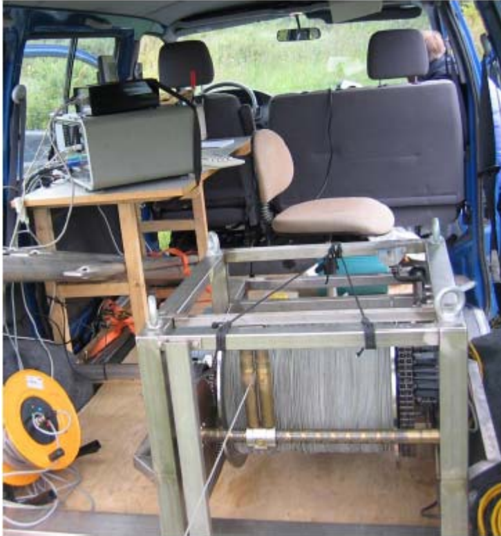
Figure B2. The logging winch is installed inside the logging car together with the electronic steering and recording unit.
