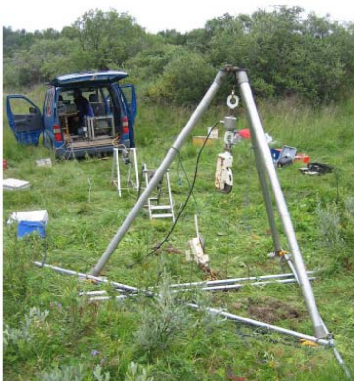
Figure B1. The temperature logging system in the field, here at Gåvålivatnet, Hjerkind.
