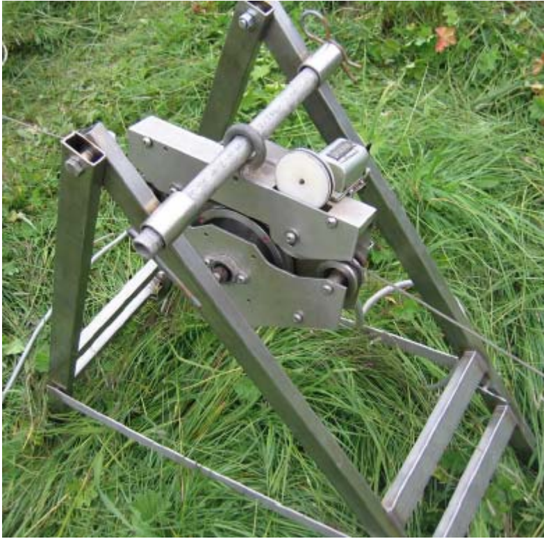
Figure B4. The electronic depth counter. An additional mechanical counter is also used (on top of the unit with the small white wheel).
