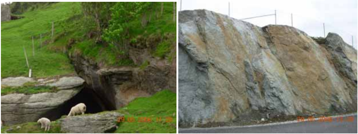
Figure 6.8. Left: NE-SW large open joints at site 2 and right: NE-SW large joints at Site 3.
