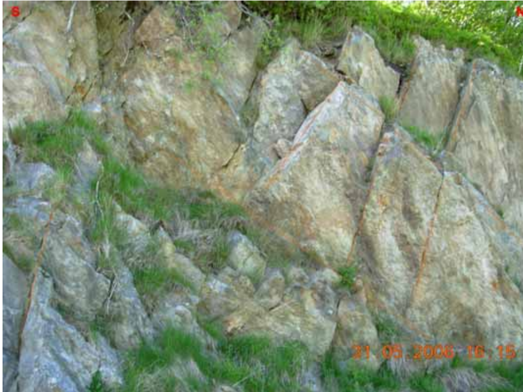
Figure 6.19. Two sets of roughly E-W striking joints forming a conjugate system with a N-dipping one and a S-dipping other one (foliation is roughly parallel to picture surface) (site 17).
