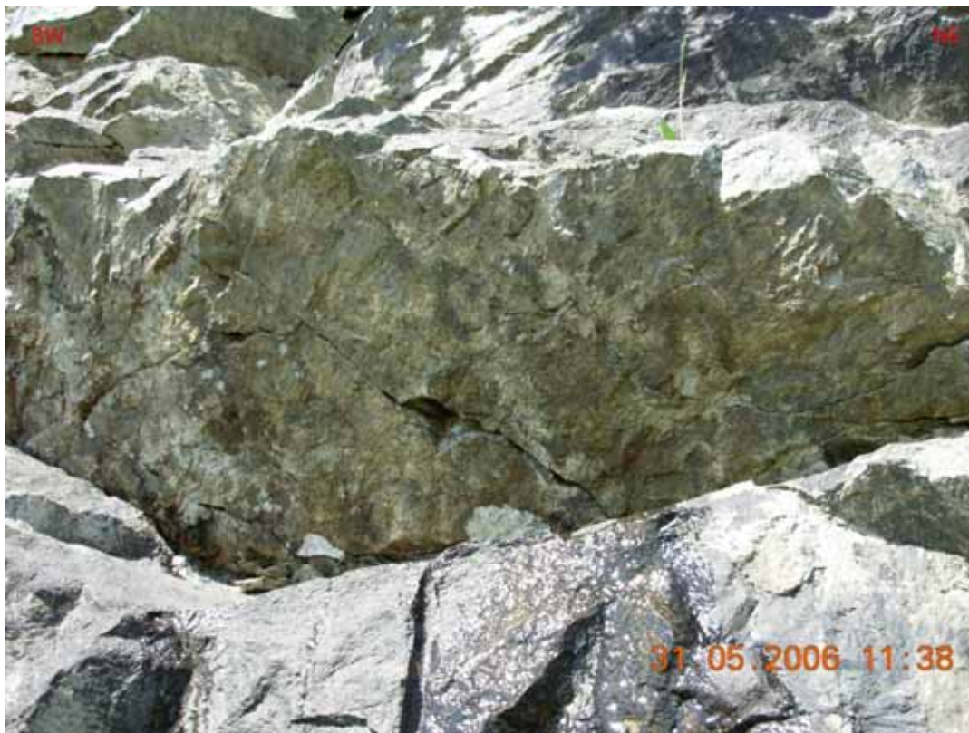
Figure 6.21. Large N-S strike-slip fault plane (site 15).
