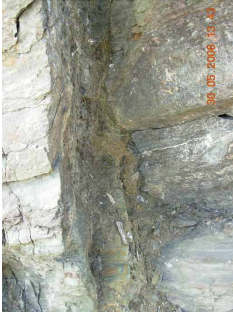
Figure 6.13. An E-W trending fault zone filled with fault rocks, 10 cm wide (site 8).
