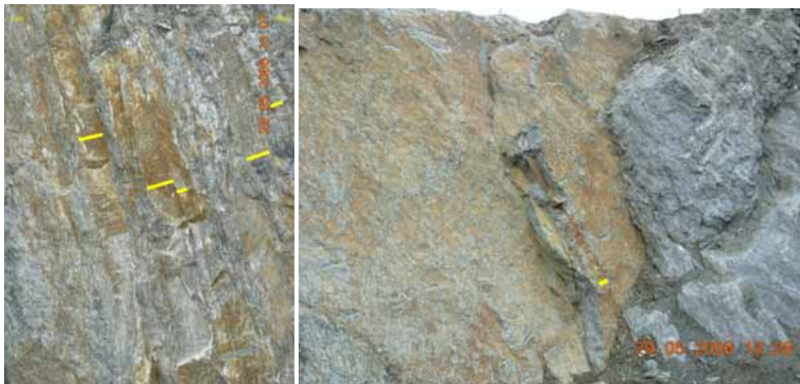
Figure 6.7. Site 3. 5 cm wide quartz-rich veins trending NW-SE, steeply dipping SW (width along yellow lines on pictures) and cutting across the fabric of the micaschist host-rock and NE-SW large joints on the right picture.
