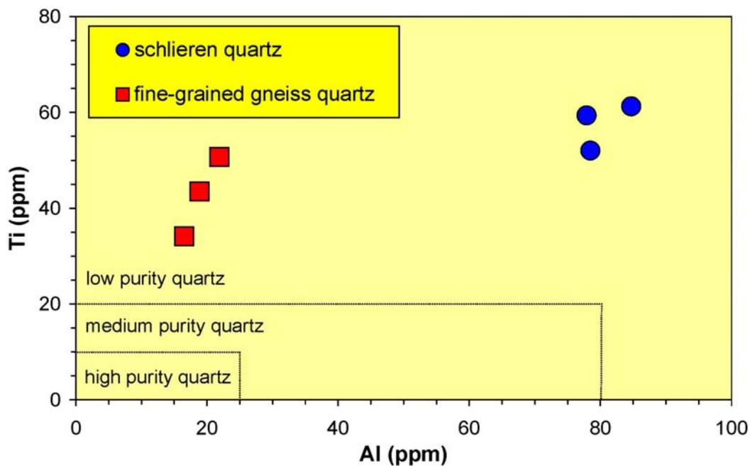
Fig. 3. Plot of Al versus Ti concentration in quartz from the Knaben locality. The high Al and the very high Ti concentration in the fine-grained gneiss quartz and schlieren quartz as well define the quartz as low quality raw material.
