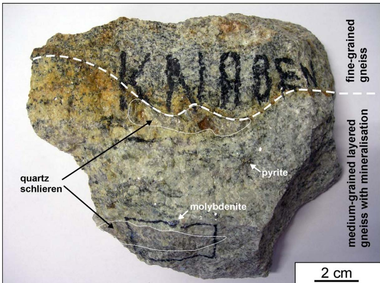
Fig. 1. Fine- to medium-grained granitic/granodioritic gneiss from the Knaben locality with molybdenite mineralisation.
