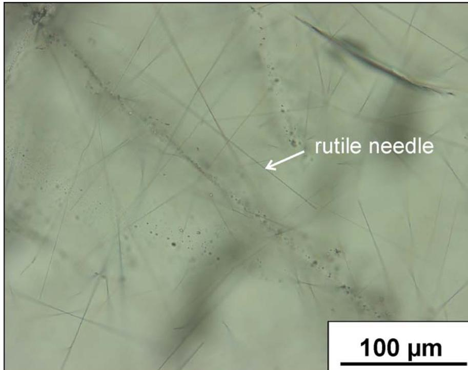
Fig. 2. Sub-microscopic inclusions of rutile needles in schlieren quartz.
