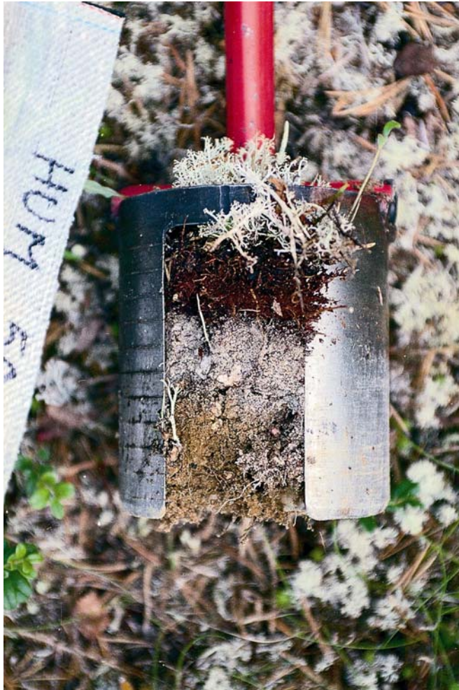
Figure 3. Sampling tool with captured humus on top of upper part of mineral soil horizons.
