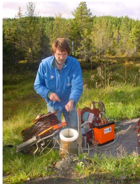
Resistivity logging of wells using the ABEM equipment.
