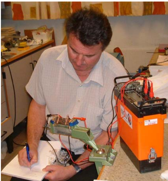
Resistivity measurements on samples in laboratory.
