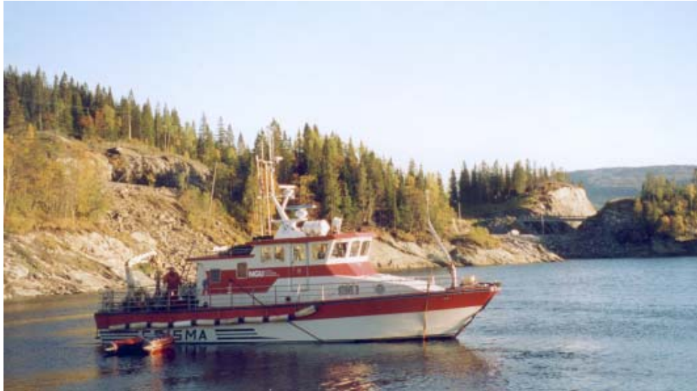
R/V "Seisma" within the slide-scar of the 1996 Finneidfjord slide. The TOPAS transducer/reciever system is strapped to the bow of the vessel when surveying.
