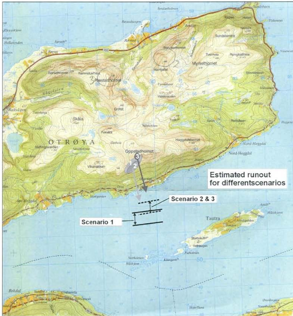
Figure 28. Estimates of possible run-out zones for three scenarios of sliding from the Oppstadhornet area. Each square of the map is 1 X 1 km in size.
