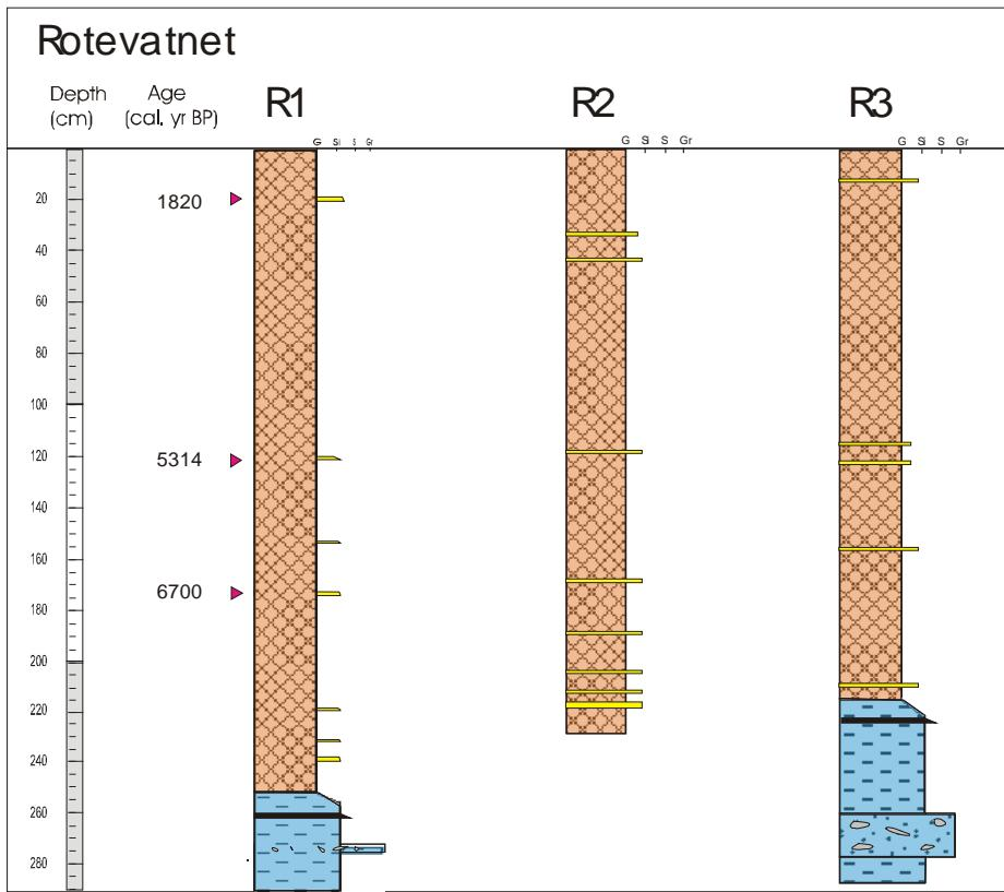
Fig. 20. Lithological logs of cores from Rotevatnet. For legend see Fig. 16.
