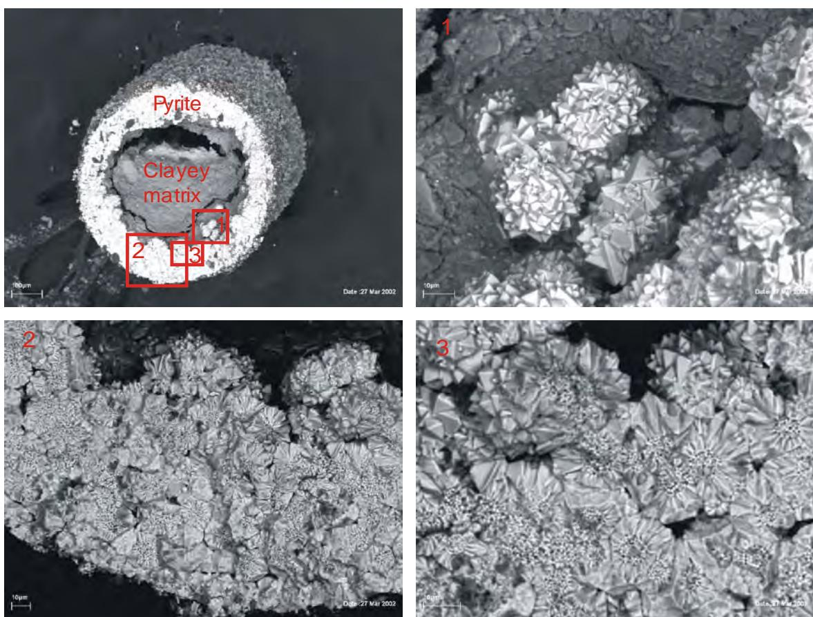
*Fig. 11. SEM-BSE (Scanning Electron Microscope BackScattered Electron) images of accumulations of authigenic frambooidal pyrite in the lower part NGU-4L/SC. Clusters of frambooidal pyrite commonly form subvertical rods and chimneys. Pyrite chimneys are occasionally filled with clayey sediment matrix. Close-ups of pyrite frambooids demonstrate different morphologies including crystalline surfaces as well as relatively smooth infilling appearances (next page).*
