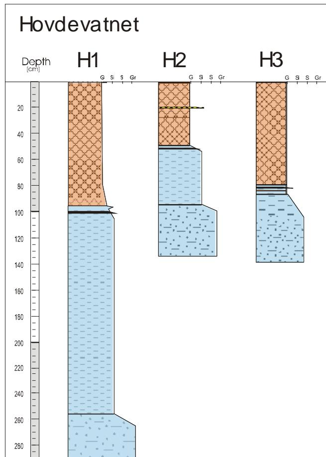
Fig. 22. Lithological logs of cores from Hovdevatnet. For legend see Fig. 16.
