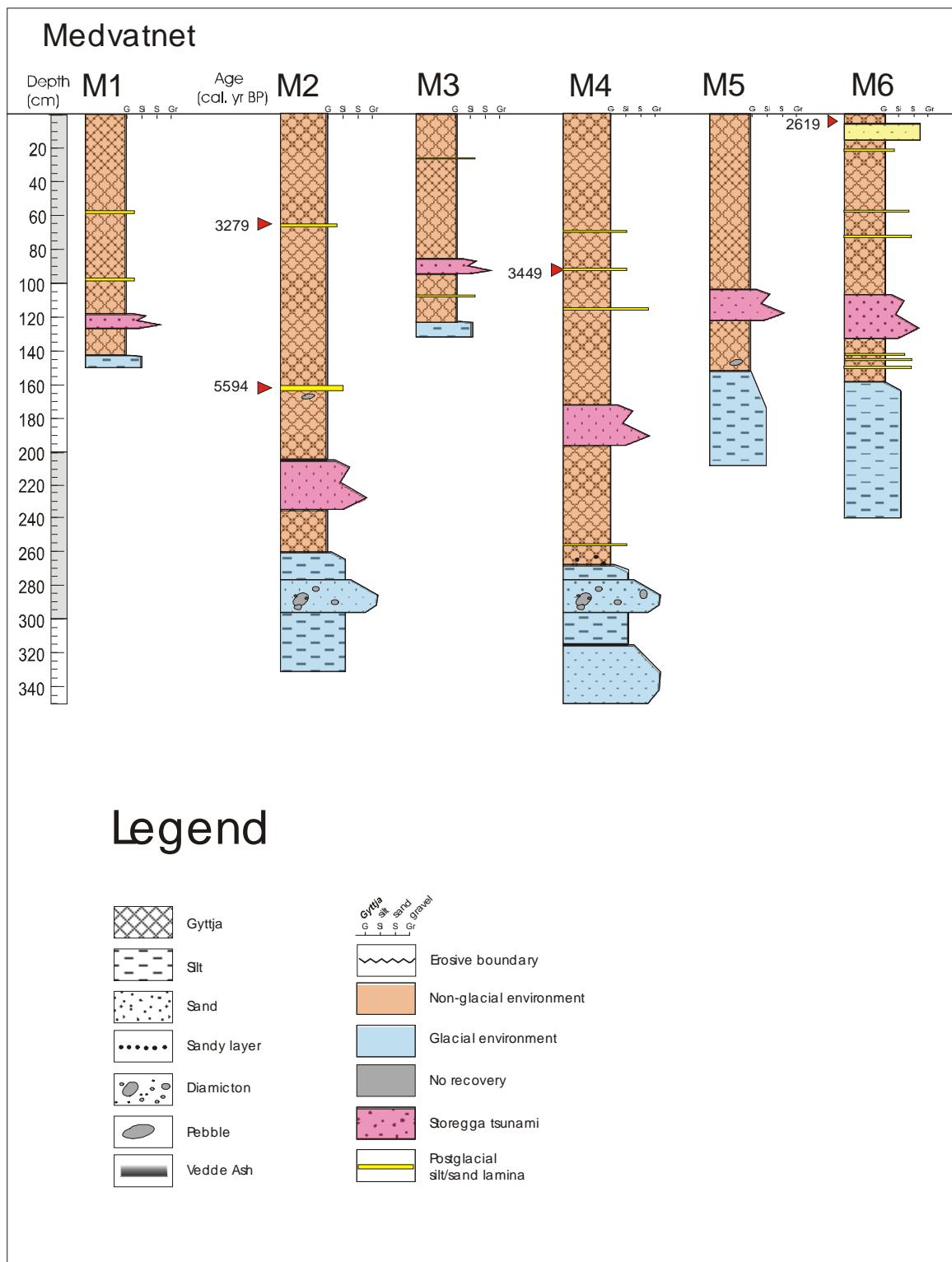
Fig. 16. Lithological logs of cores from Medvatnet.
