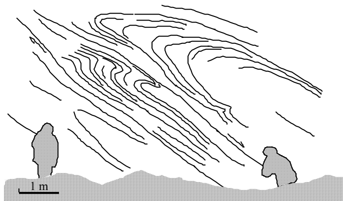
Fig. I 1.6. Drag fols in the EGOG foliated margin. The central part of the EGOG massif is on the left of the photo and the foliation is dipping to the south.
