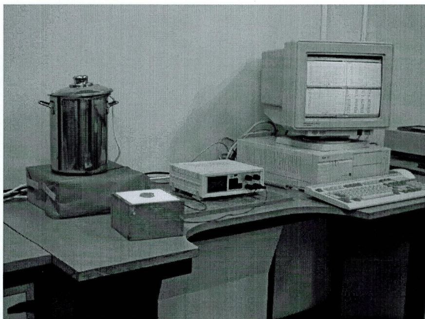
Figure 2. Thermal conductivity apparatus at NGU.
