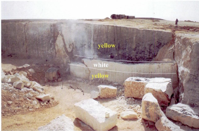
Fig. 2. ISO Marble limestone quarry, Sheikh Fadl. Distribution of limestone types in the quarry is shown on the photo.
