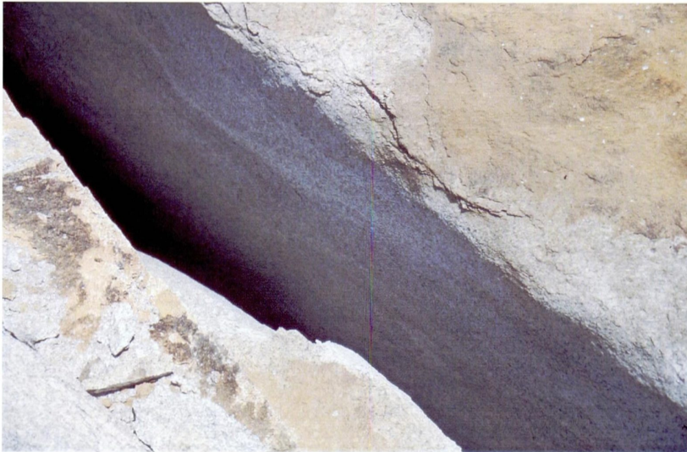
Fig. 12. Diffuse grey-white banding in white granite, Heimar deposit in a flame torch channel (site 1). The channel is appr. 20 cm wide.
