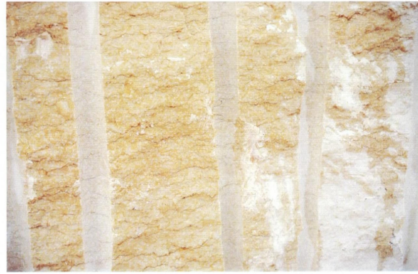
Fig. 3. Typical section of yellow, attractive limestone in the ISO Marble quarry, Sheikh Fadl (wet, rough surface). Diametre of drill holes are appr. 35 mm.
