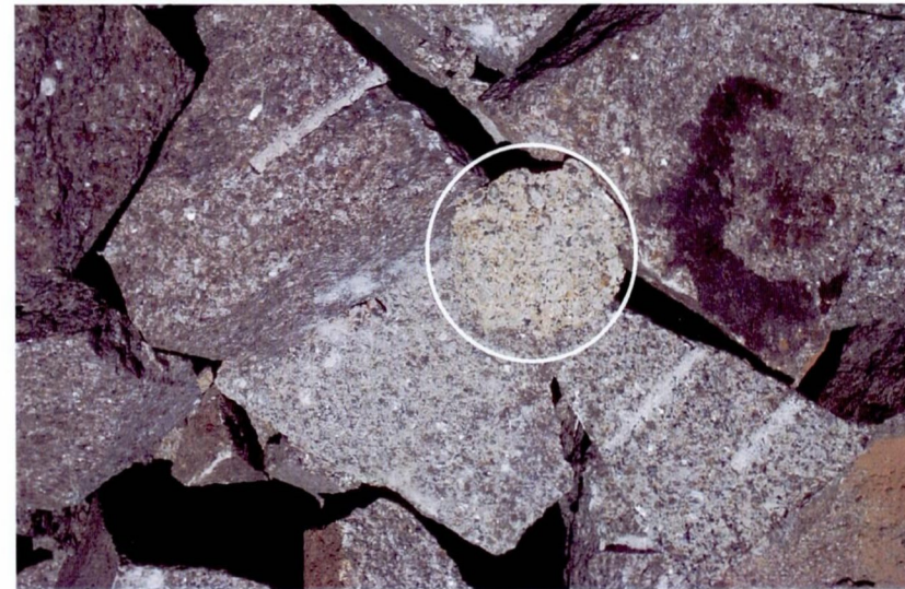
Fig. 5. Colour difference between yellow granite from the 'Mohammed-quarry' (centre, marked by white line) and typical samples from the Hadidsolb 2 deposit. Diameter of the white circle is appr. 20 cm.
