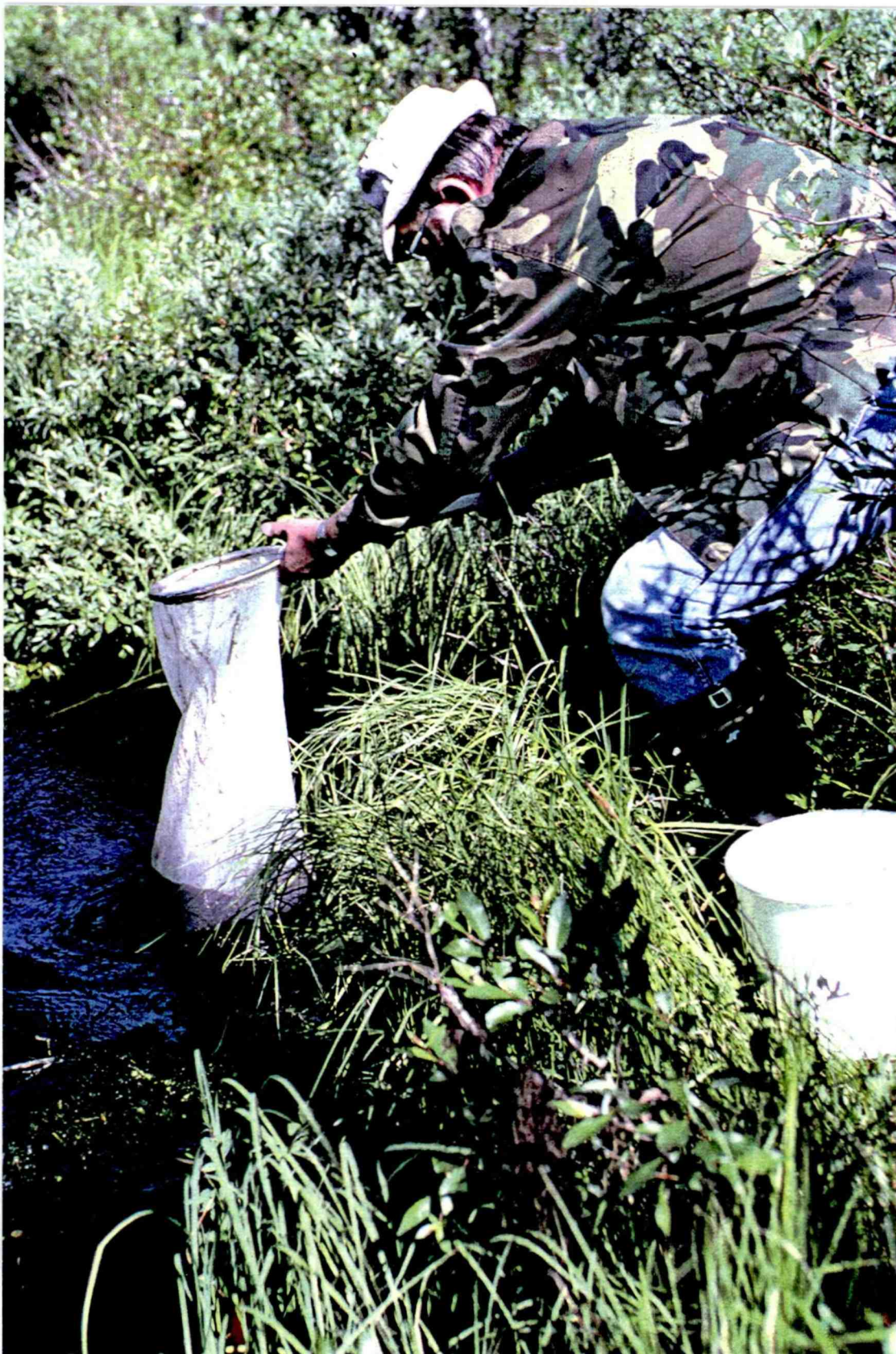
Fig. 4: Sampling of organic stream sediments. Photo: Clemens Reimann, NGU
