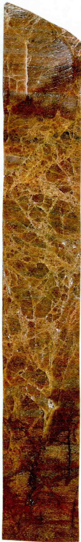
Fig. 5. Photograph of polished sample from the brecciated reddish-grey quartzite at 33 m depth. The diameter of the core is 34 mm.
