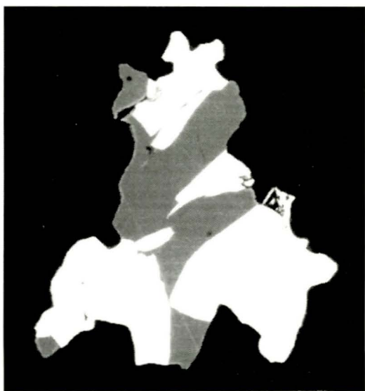
Fig. 2. SEM back-scattered electron image of rutile (grey) and ilmenite (white) intergrowth from the Husebø eclogite at Holsnøy, Bergen Arcs. Photo width 0,2 mm.
