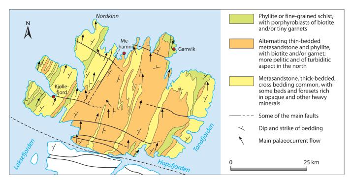
Figure 5. Simplified geological map of Nordkinn Peninsula showing palaeocurrent flow as measured in cross-bedded sandstones (corrected for dip of bedding and fold plunge).
