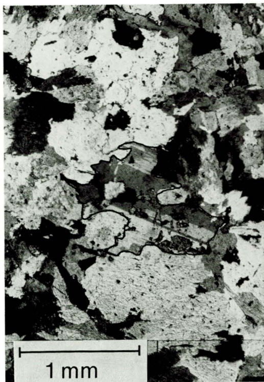
Fig. 4. complete deuteric/low-grade metamorphic alteration of orthopyroxene and clinopyroxene to light actinolite. Plagioclase has been altered to chessboard albite (outlined).
