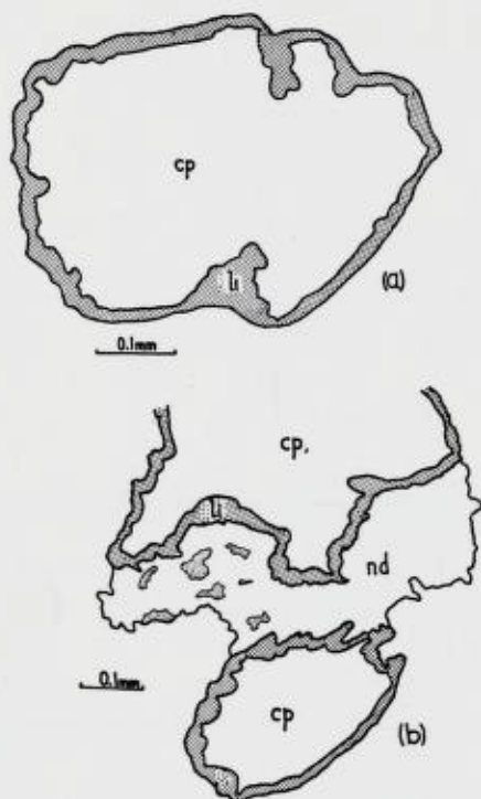
Fig. 2. Replacement rims of secondary limonite (li) around grains of chalcopyrite (cp). Note the absence of such rims at the grain-boundaries of the neodigenite (nd). Finely stippled areas in the neodigenite are replacement remnants of bornite.
