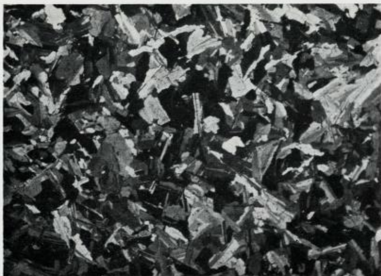
Fig. 1. Leucodiabas med nesten bare albitt. 15 \times . Leucodiabase consisting nearly exclusively of albite. \times 15.
