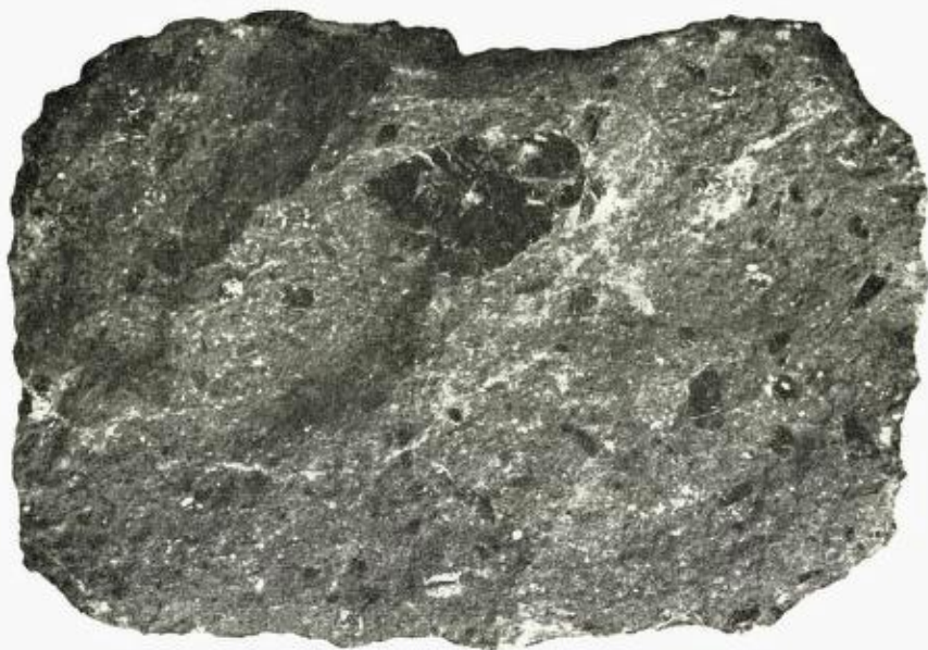
Fig. 2. Biotite lamprophyre. Hand specimen. \frac{3}{4} nat. size.
