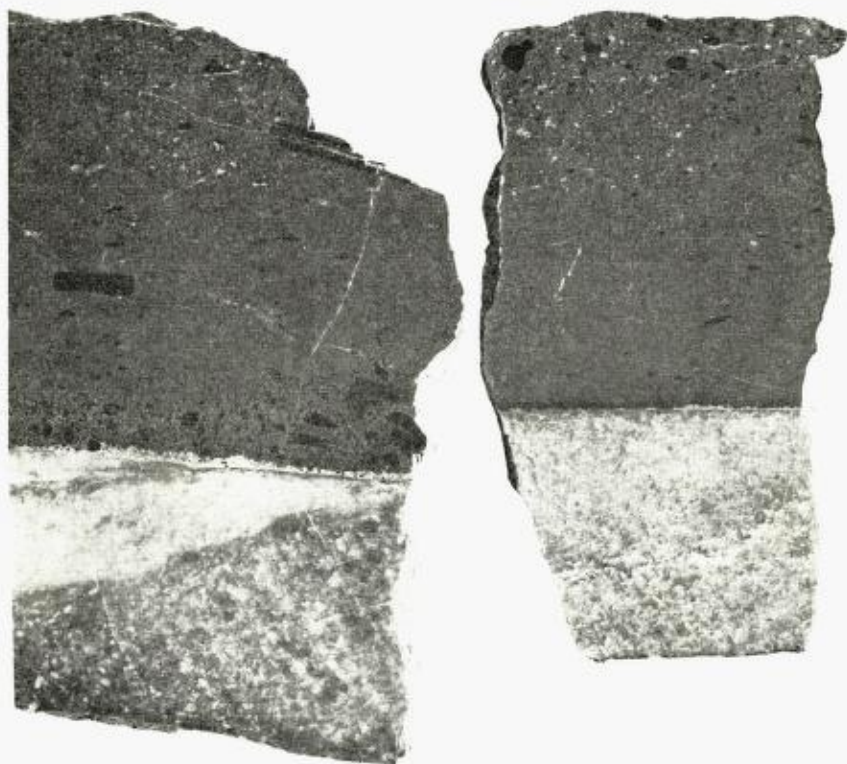
Fig. 3. Biotite lamprophyre — limestone contacts. Polished specimens. \frac{1}{2} nat. size. The left picture (a) shows the porphyritic border facies, 15 mm wide. «Anomalous» large inlets of biotite above the discontinuity. To the right (b) is demonstrated fine-grained chilled margin and increase in the size and amount of phenocrysts from the contact. The white contact layer is seen in both pictures.
