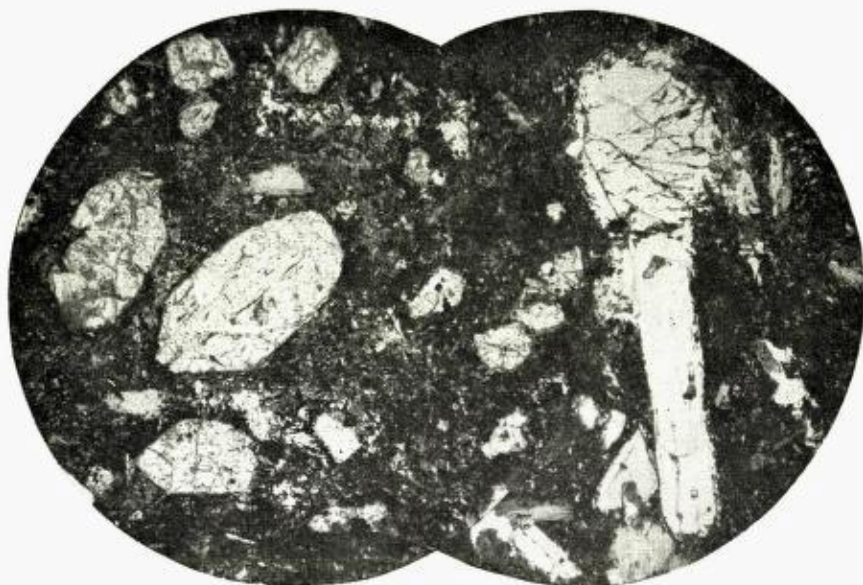
Fig. 4. Biotite lamprophyre. Photomicrographs, 26 X. Right: Phenocryst of biotite contiguous to an analcite ocellus. Left: Pseudomorphs after olivine.
