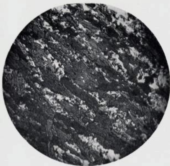
Plate I. Amphibolite, specimen 2448 c. Plane polarised light. Green hornblende in a fine grained groundmass of plagioclase and quartz. Diam. of photo = 2 mm.
