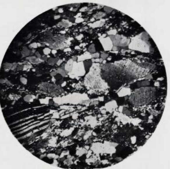
Plate II b). Mylonitic gneiss, specimen 547. Crossed nicols. Crushed, fine grained groundmass of quartz and feldspar. A few large, highly cataclastic plagioclase grains. Diam. of photo = 2 mm.
