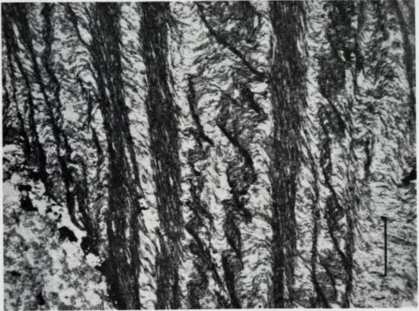
Fig. 3. Black phyllite of fig. 2 showing detail of differentiation structure and its folding. Scale mark 0.5 mm.
