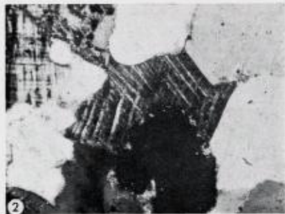
Plate 3 Fig. 1. Rounded quartz grains with secondary overgrowths. "Hyalithes Zone" feldspathic sandstone. Crossed polarisers. X33.
