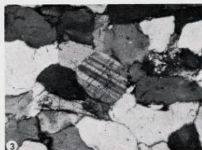
Plate 3 Fig. 3. Rounded feldspar grain projecting into adjacent quartz grains. Feldspathic sandstone of the "Hyalithes Zone". Crossed polarisers. X94.
