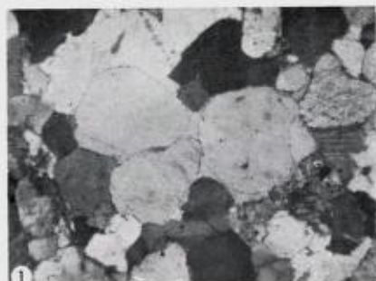
Plate 3 Fig. 1. Rounded quartz grains with secondary overgrowths. "Hyalithes Zone" feldspathic sandstone. Crossed polarisers. X33.
