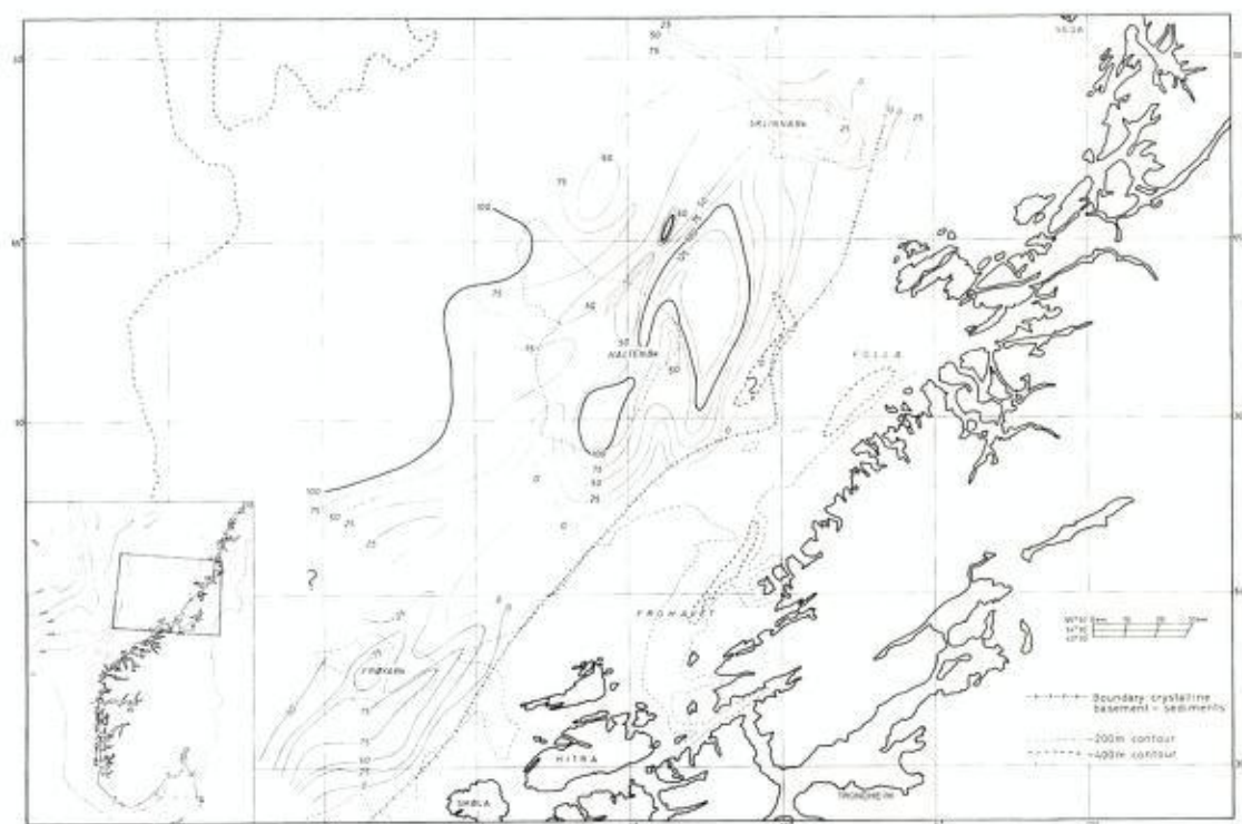
Fig. 1. Variation in thickness of Quaternary sediments off the coast of Trøndelag and Nordland. Contours in milliseconds. (Eldholm & Nysæther, 1969.)
