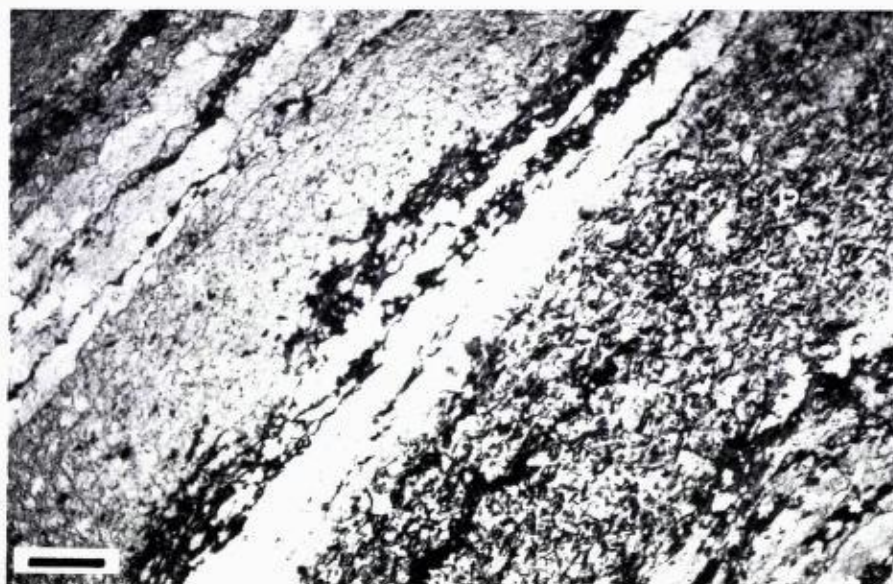
Fig. 4. Augen gneiss of Fig. 3. Note the zoisite needles in lens of fine-grained plagioclase (P). No zoisite in lens of fine grained K-feldspar (K). Bar scale = 0.1 mm. Plane-polarised light.
