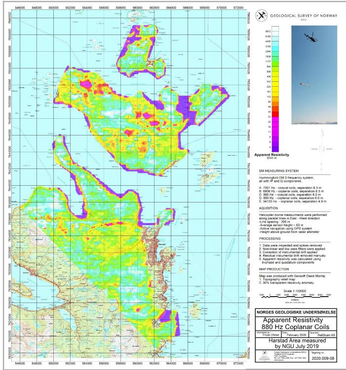
Figure 12: Apparent Resistivity. Frequency 880 Hz, Coplanar coils
