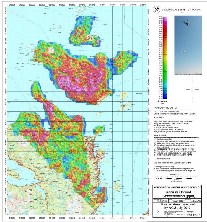
Figure 16: Uranium ground concentration
