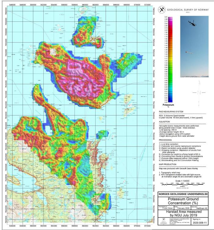
Figure 15: Potassium ground concentration
