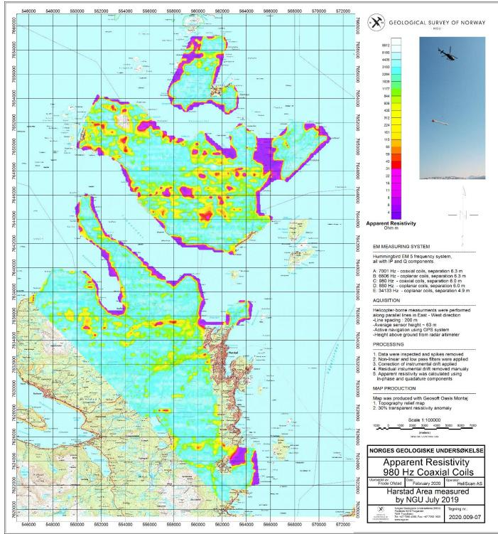
Figure 11: Apparent Resistivity. Frequency 980 Hz, Coaxial coils
