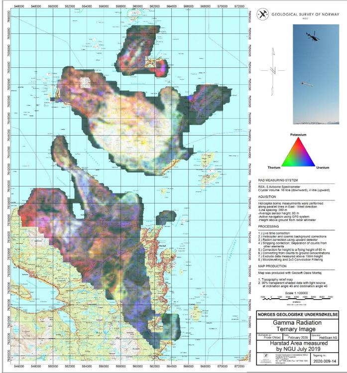
Figure 18: Radiometric Ternary Image
