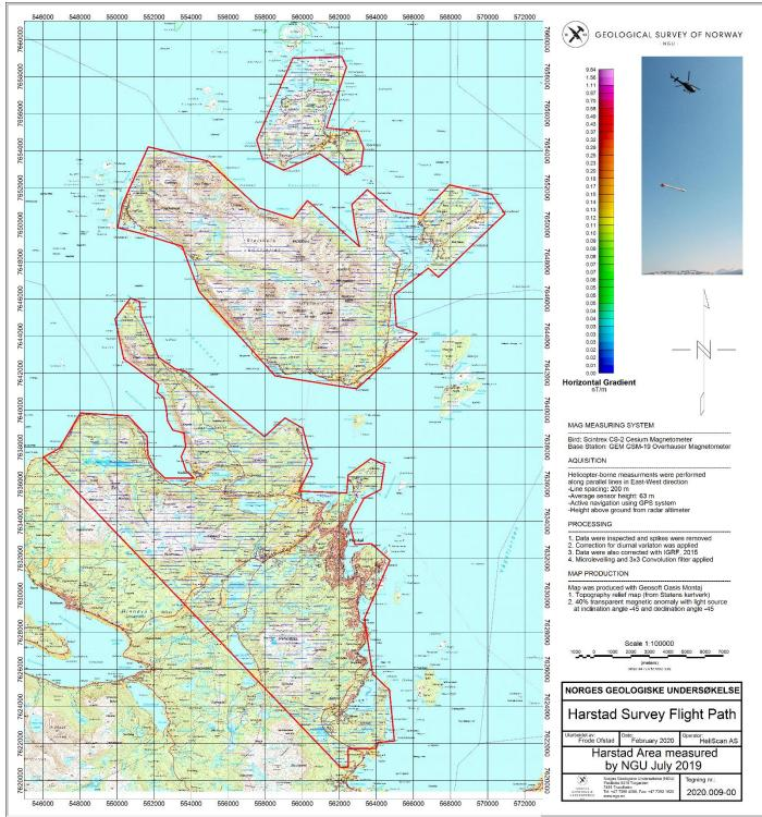
Figure 4: Harstad survey area with flight path
