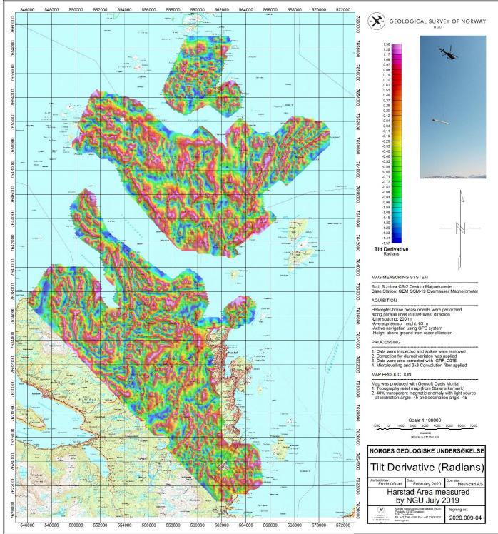
Figure 8: Magnetic Tilt Derivative
