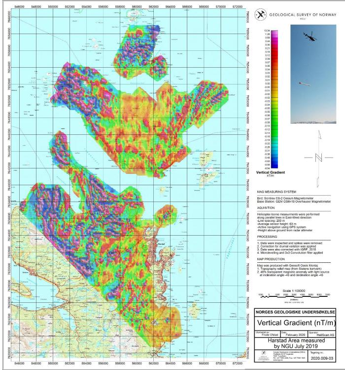
Figure 7: Magnetic Vertical Gradient
