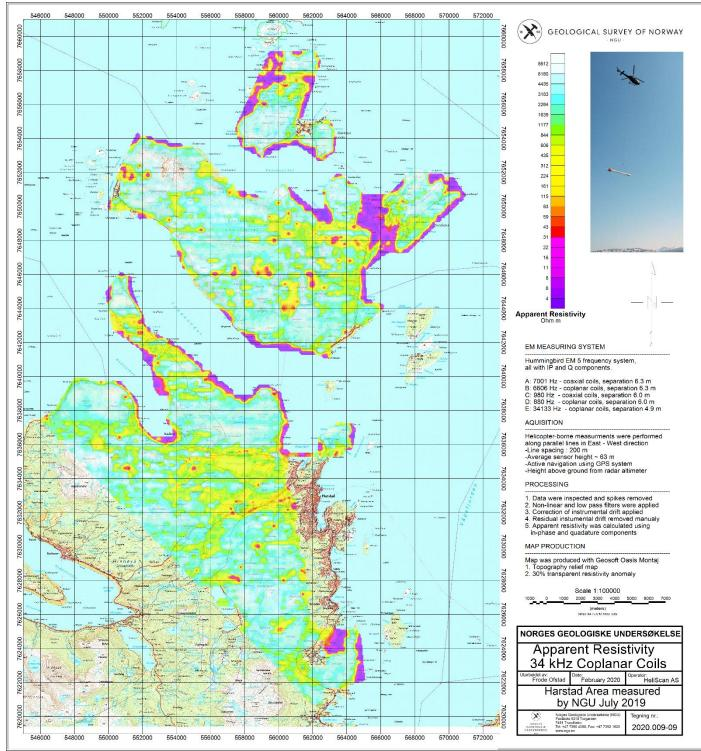
Figure 13: Apparent Resistivity. Frequency 34133 Hz, Coplanar coils
