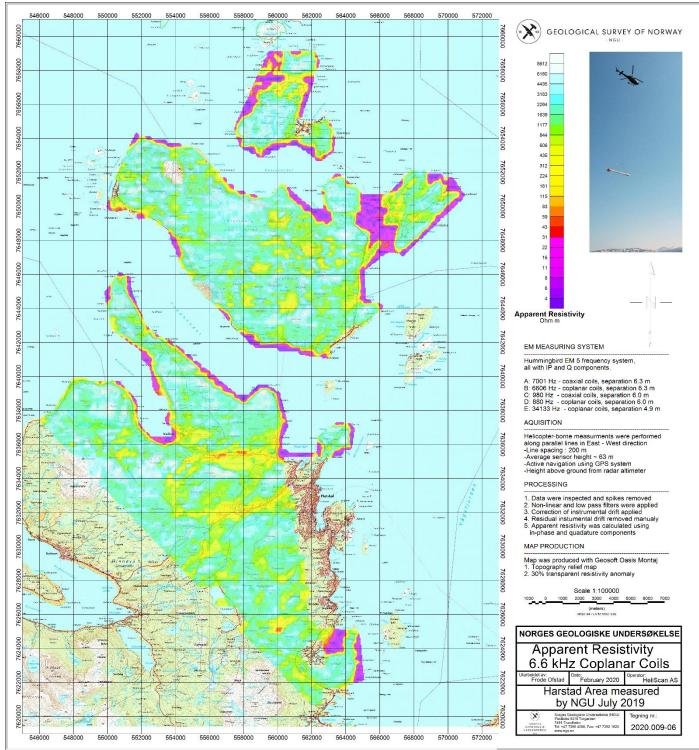
Figure 10: Apparent Resistivity. Frequency 6600 Hz, Coplanar coils
