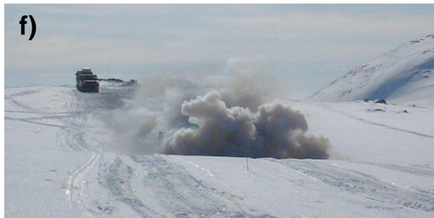
Figure 1. Pictures from the field work. a) From the western line at Sennalandet. b) From the western line at Masi. c) Working with the snowstreamer at the drum. d) Node for recording. e) and f) Shots made with detonating cord.
