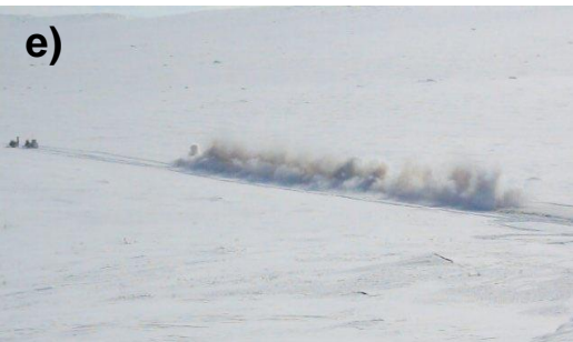
Figure 1. Pictures from the field work. a) From the western line at Sennalandet. b) From the western line at Masi. c) Working with the snowstreamer at the drum. d) Node for recording. e) and f) Shots made with detonating cord.
