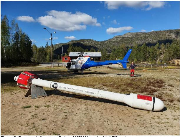
Figure 2: Pegasus helicopter, pilot, and NGU Hummingbird EM system
