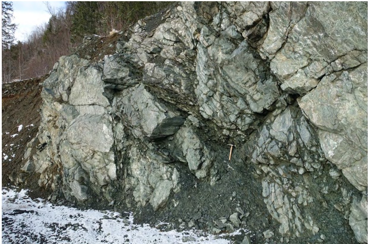
Figure 8.7. Deep weathering in greenstone at the Lia Pukkverk locality; sample numbers 108520 and -21.
