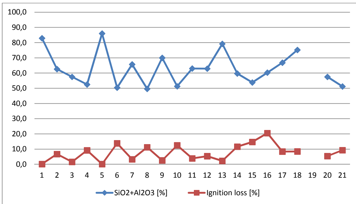
Figure 8.28. XRF data in weight%. Variation of \text{SiO}_2 + \text{Al}_2\text{O}_3 and Ignition loss, for all samples 108601 through to 108521. The numbers along the x-axis correspond to the last integers in the sample numbers. \text{SiO}_2 + \text{Al}_2\text{O}_3 is seen to be much higher for the fresh rocks (odd numbers) compared to their respective weathered ones (even numbers, except samples 108517 and 108521 that are also weathered samples). The ignition loss shows higher values for the weathered samples (also demonstrated in Figure 8.26).
