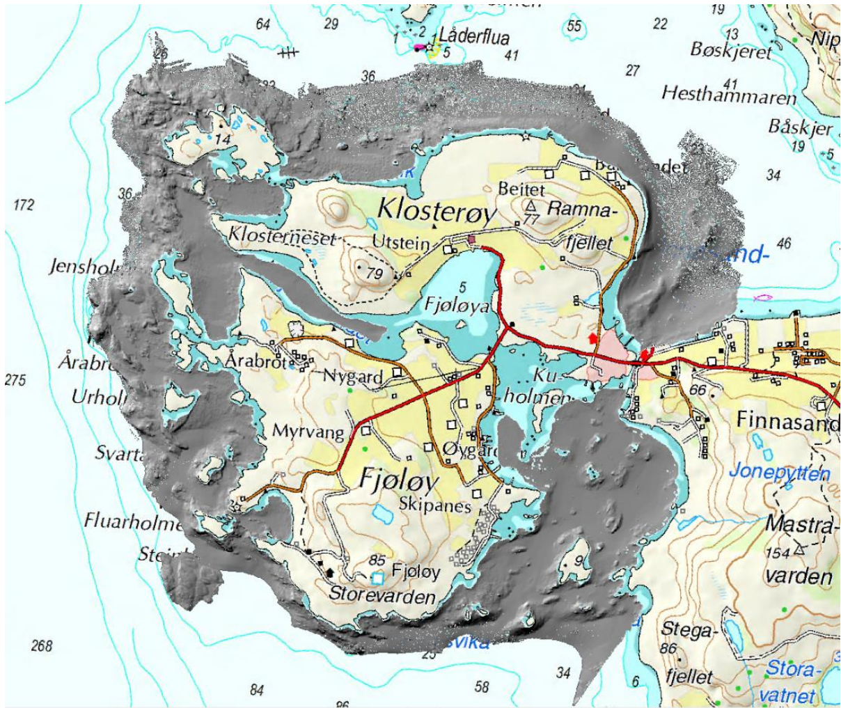
Figure 7.1. Shaded relief terrain model (grid size 20 cm) of the MBES data acquired by the Norwegian Mapping Authority in 2020.
