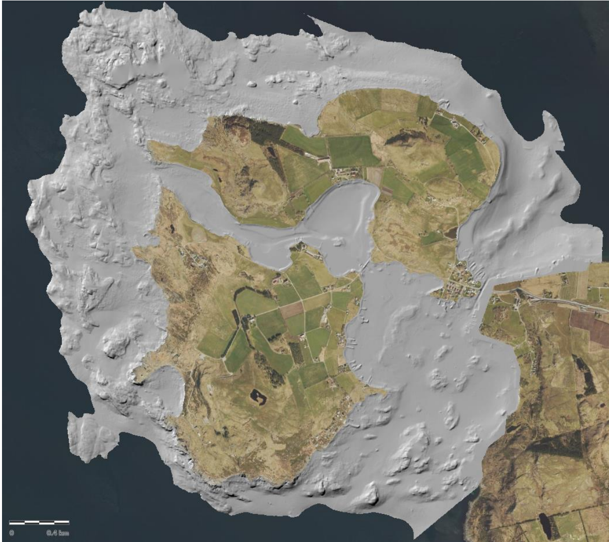
Figure 4.5. Shaded relief showing the bathymetric coverage of the Field LIDAR dataset. Figure from høydedata.no (Kartverket, 2023).
