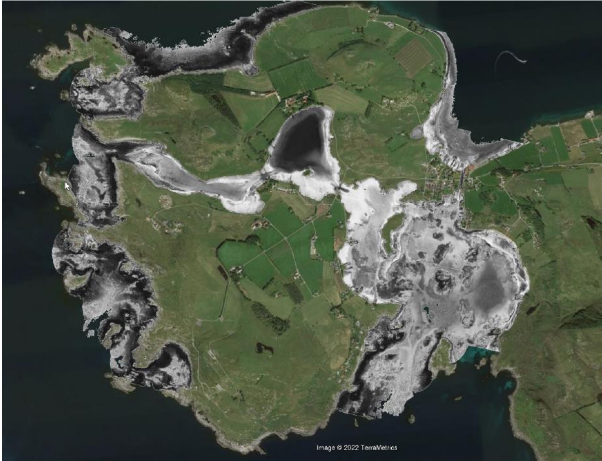
Figure 4.3. Depth-normalized intensity from Hexagon LIDAR survey. Figure copied from Hexagon (2022).
