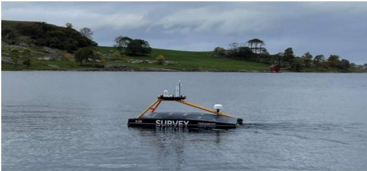
Figure 7.5. The XOCEAN XO-450 USV during mapping of priority area 3, October 26th, 2021
