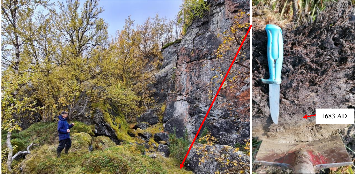
Fig. 26. A (left): Blocks of rock fallen from an up to 20 m high bedrock wall in the uppermost part of the unstable bedrock slope shown in figure 25. B (right): A sample of plant remains was taken from the base (at the knife edge point) of the thickest surficial peat between rock boulders, indicated by red arrow, in front of the adjacent collapsed bedrock backwall shown to the left. A ^{14}\text{C} -dating of these plant remains indicate that the bedrock wall collapses probably occurred before 1683 AD (Table 4; no. 75).
